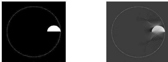
Fig. 2.11. A smaller semi-circular phantom and its reconstruction for T = 4 with the “crater” trapping speed. There is a noticeable blurring on the circular boundary at the point where the normal ray is trapped (i.e., where the circle is tangential to the radius).
