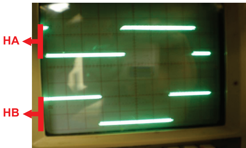
Fig. 4-16 Hall Outputs Successfully Generated
