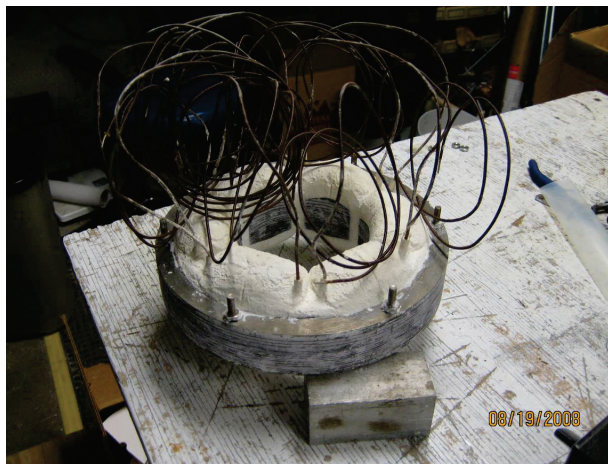
Fig. 2-8 Motor Stator after Curing
