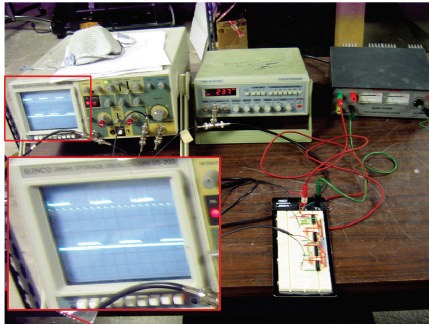
Fig. 3-22 Test of Digital Circuit Using Function Generator
