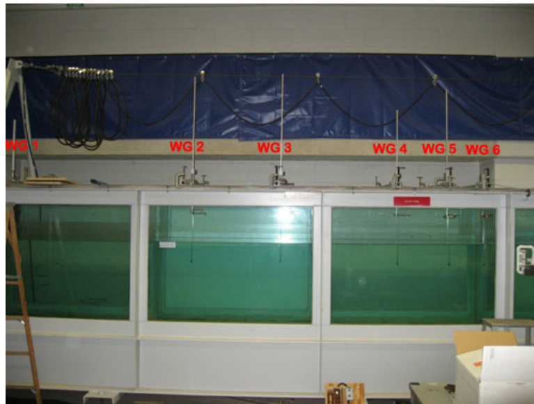
Fig. 5.5 Measurement locations of six wave gauges.
