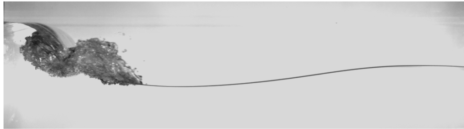
(b) t = 0.11 s (a small local crest between the two clockwise rollers)
