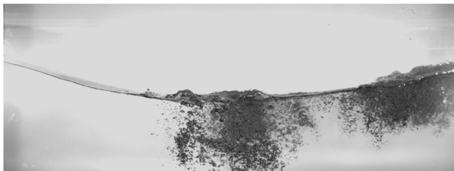
(m) t = 0.99 s (the 1 st impinging roller going down to z = -0.32h )
