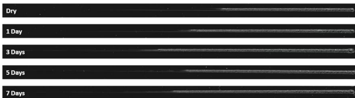
Figure 6.6 Digitally scanned images of SAN 27 periodically scratch tested after being exposed to a humid environment. (Resolution = 300 dpi)
