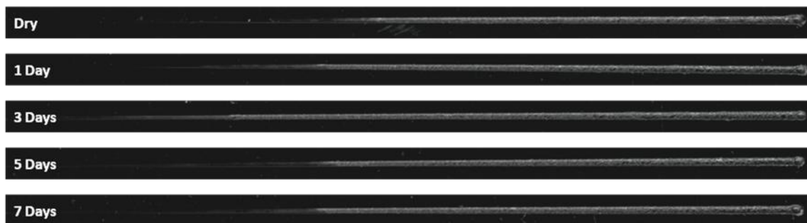
Figure 6.5 Digitally scanned images of SAN 19 periodically scratch tested after being exposed to a humid environment. (Resolution = 300 dpi)
