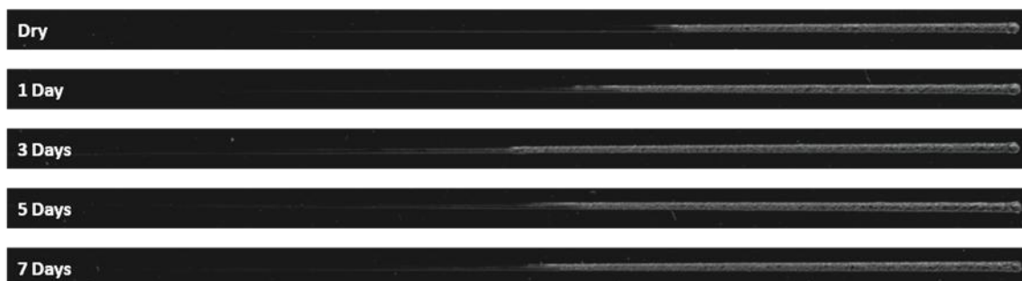
Figure 6.7 Digitally scanned images of SAN 35 periodically scratch tested after being exposed to a humid environment. (Resolution = 300 dpi)
