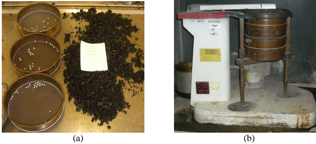
Figure 7: (a) Loose sample on the right, before being sieved through the set of sieves on the left, equipped with stainless steel balls. (b) Mechanical sieving being performed.
