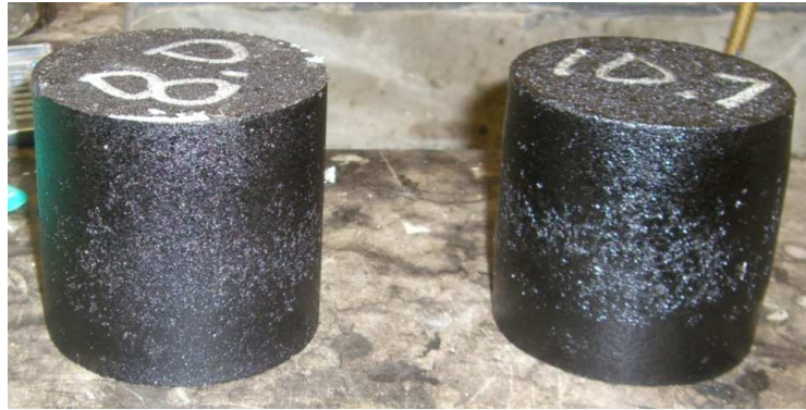
Figure 12: Two limestone SGC specimens prepared with different asphalt contents. The one on the right has crept under its own weight, resulting in a slight “barrel” shape.
