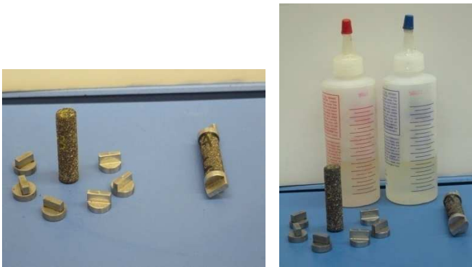
FIGURE B.2 —Holders, Glue, and Specimens in the Gluing Process
