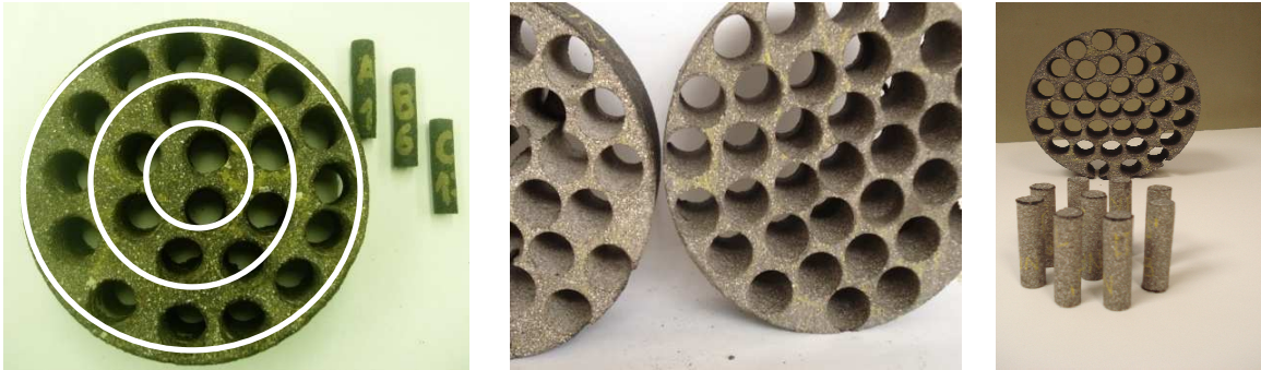
FIGURE A.4 —Coring DMA Specimens
