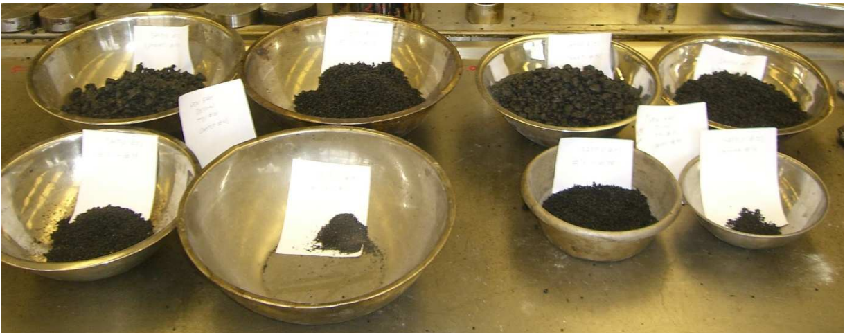
Figure 8: Two samples after sieving is completed. Four fractions are obtained for each sample.
