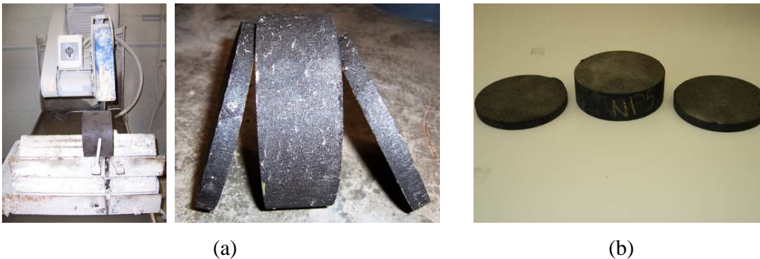
FIGURE A.3 —Sawing Process (a) and Final Result (b)
