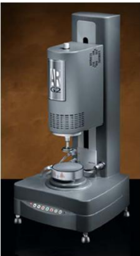
Fig. 10. AR-G2 rheometer Courtesy of TA Instrument
