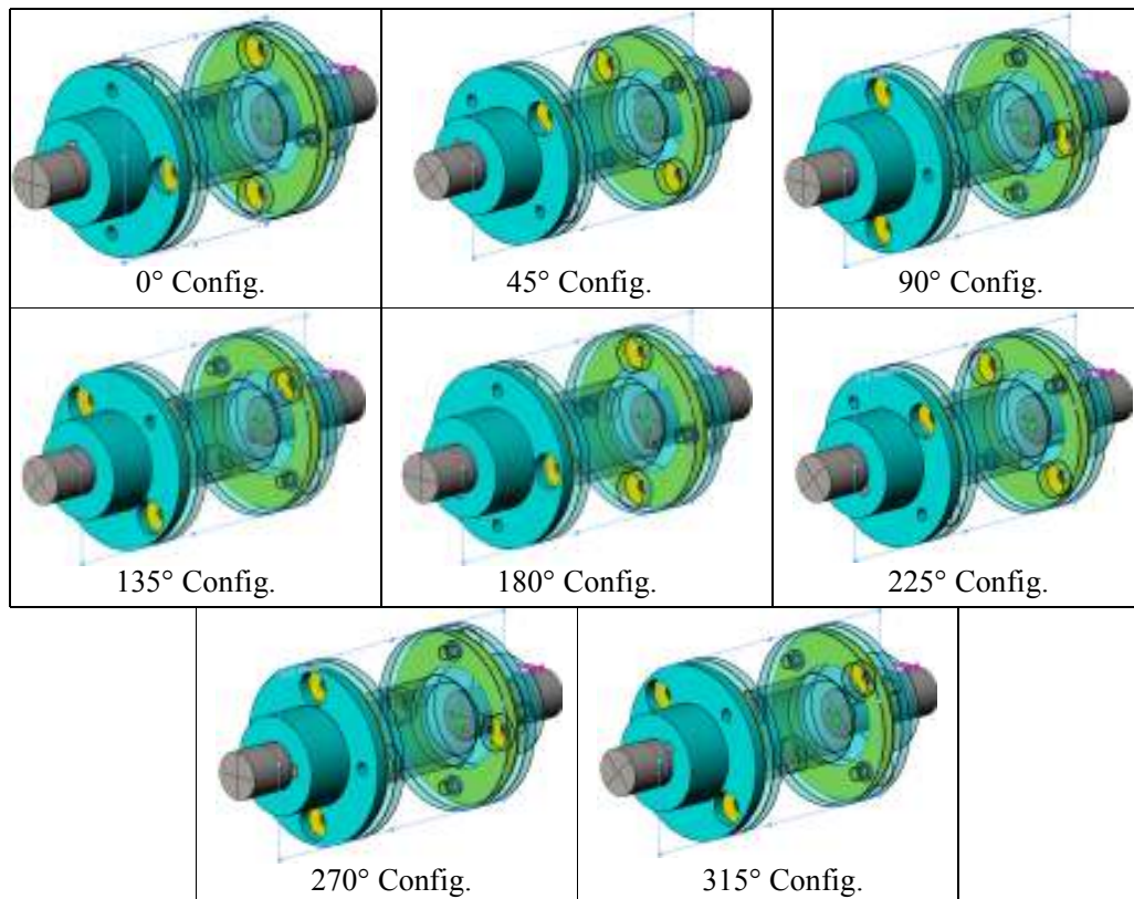
Figure 22. Eight configurations of the 4-bolt model used to simulate misalignment.
