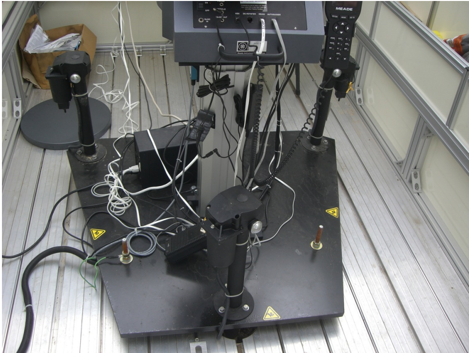
Fig. 37. Pier-tech mobile telescope pier isolated from the trailer
