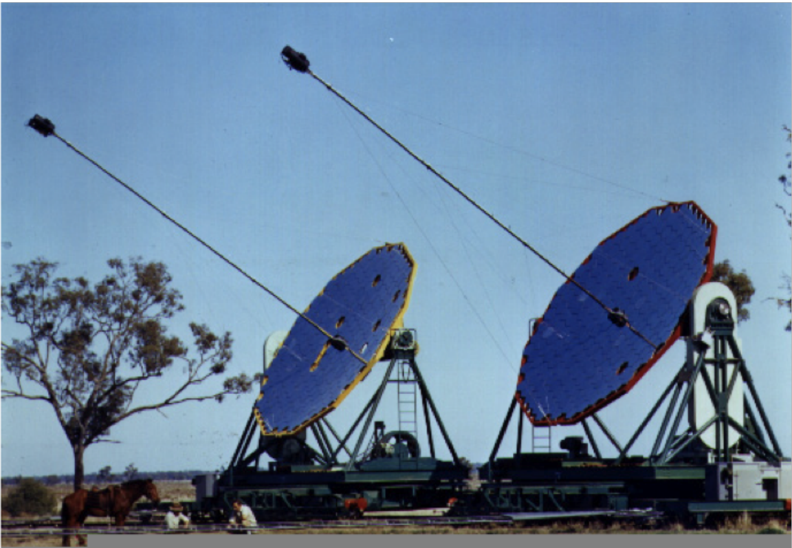
Fig. 4. Optical reflectors used in the Narrabri intensity interferometer
