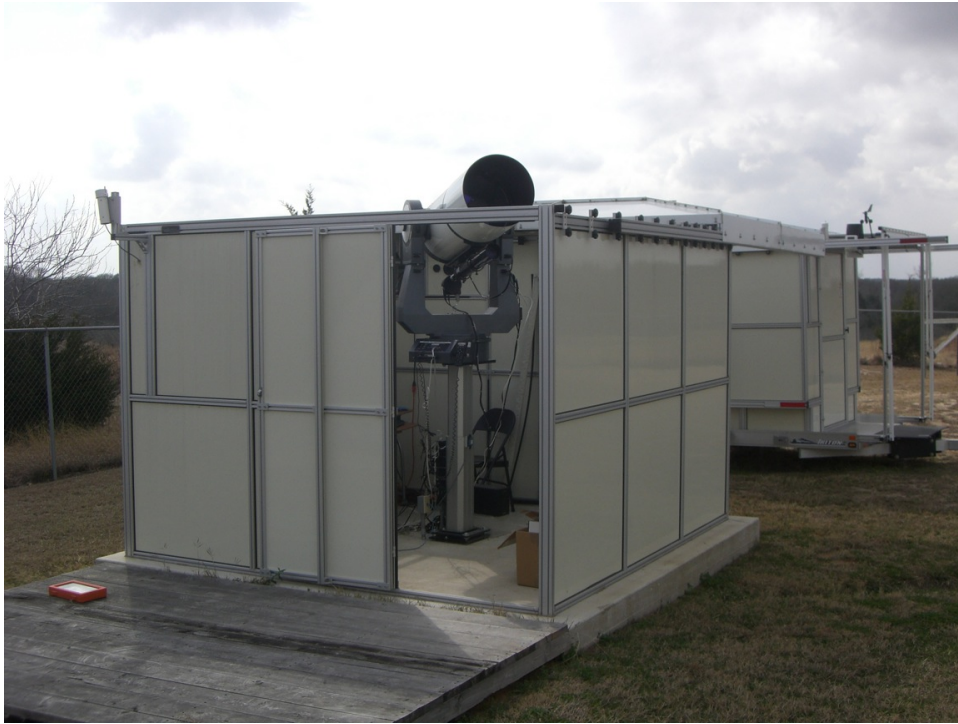
Fig. 33. Pier-tech telescope shelter
