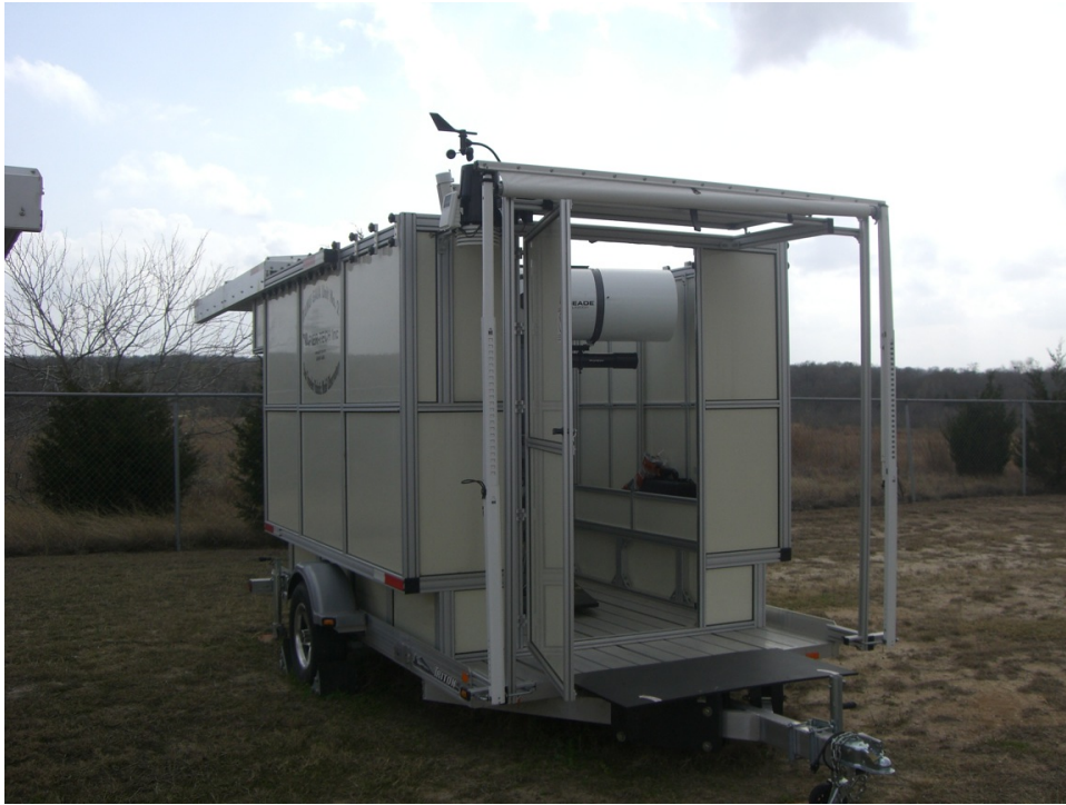
Fig. 35. Pier-tech mobile telescope shelter
