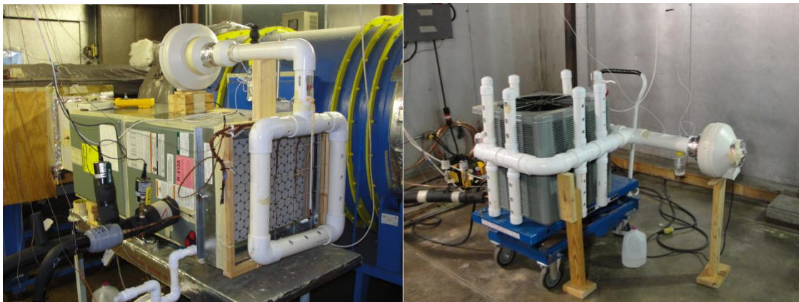
Figure 4. Photograph of the indoor room and outdoor room psychrometric stations.
