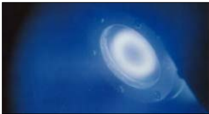
FIG. 2.6 Race course track and plasma during sputtering.
