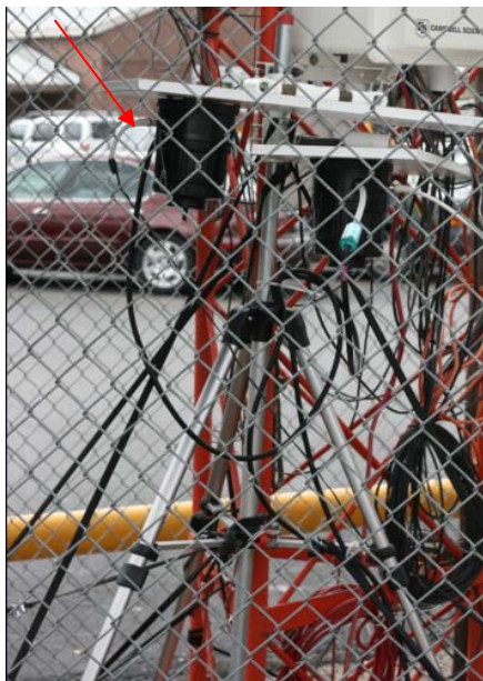
Figure 6: (a) Pictures of PIXE Streakers setup in field site and (b) Cross-sectional view of PIXE Streaker sampler configured for two size-fraction operation. Arrows indicate airflow. Air passes through the non-rotating pre-impaction stage A, where particles larger than 10 \mu\text{m} are deposited. The air then flows through an impactor slit B where particles larger than 2.5 \mu\text{m} are deposited on a moving filter. Next the air flows through the rotating filter stage C where particles smaller than 2.5 \mu\text{m} are deposited ( http://www.pixeintl.com/Streaker.asp ).
