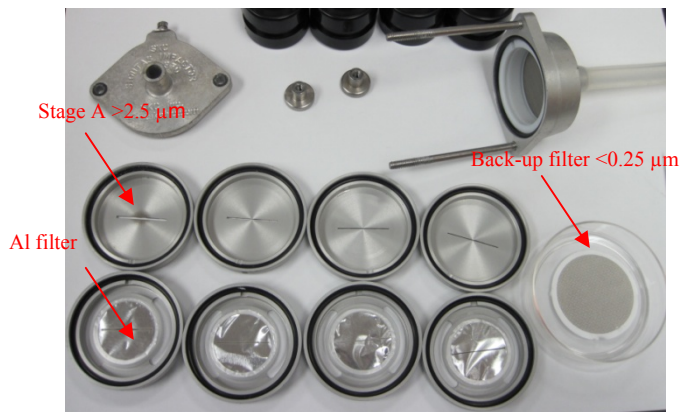
Figure 3: Pictures of the Cascade Impactor Sampler with collected particulate on aluminum filters.
