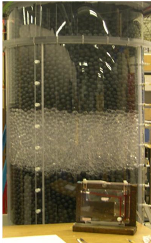
Fig. 39. A diagram and a picture of annular packed bed.
