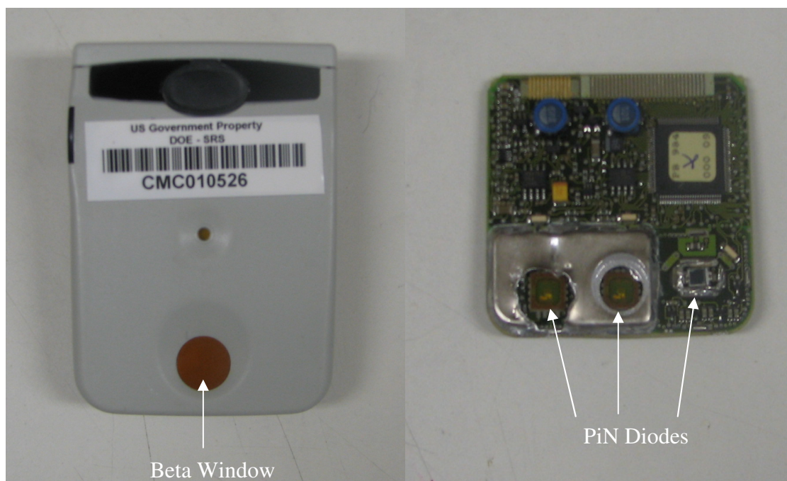
Figure 6. Front view of a Thermo MK2 electronic personal dosimeter (left). Disassembled view; the compensating case was removed on the far left diode for illustrative purposes. Note the three PiN diodes and their various shielding configurations (right).
