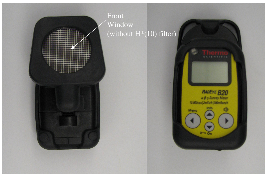
Figure 4. Front view of the Thermo RadEye B20. The H*(10) filter is not shown in this figure, but it fastens over the front window (left). Back view (right).
