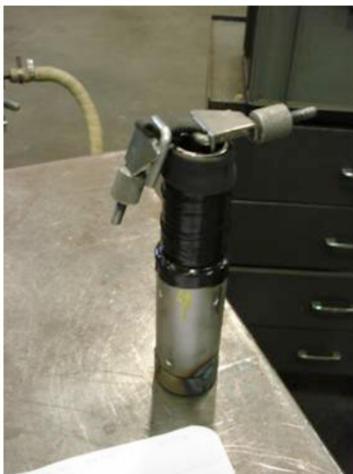
Fig. 2. Sample with crimped hose after evacuation.
