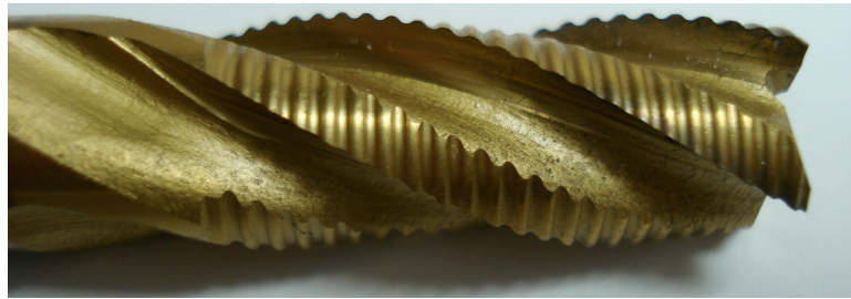
Fig. 9. Cutting tool for Nb chip formation.
