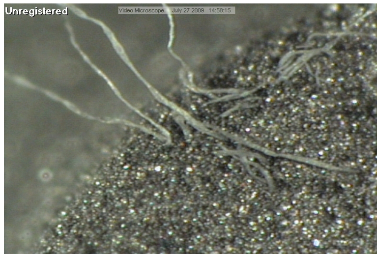
Fig. 4. Fibers embedded in Nb bulk.
