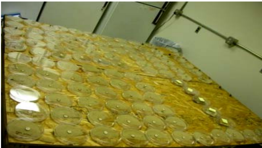
Fig. 3. An array of replicated no-choice arenas with pecan wood wafers and 250 Formosan termites.
