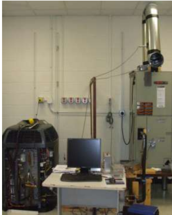
Fig. 3.1 3-Ton residential air conditioner from Trane
