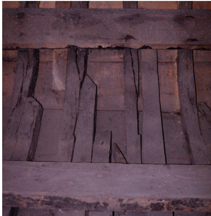
Fig. 5.1. An interior view of Kadırga showing some of the ship's hook scarves. Photo by Erkut Arcaç, courtesy of the Kadırga project (INA).
