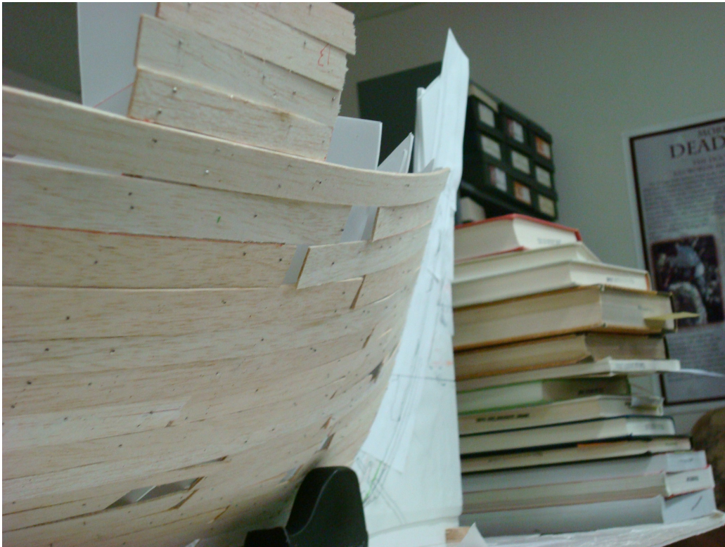
Fig. 4.9. The stern of the model showing the wale in place. The wale is the uppermost complete strake. Photo by Matthew Labbe.
