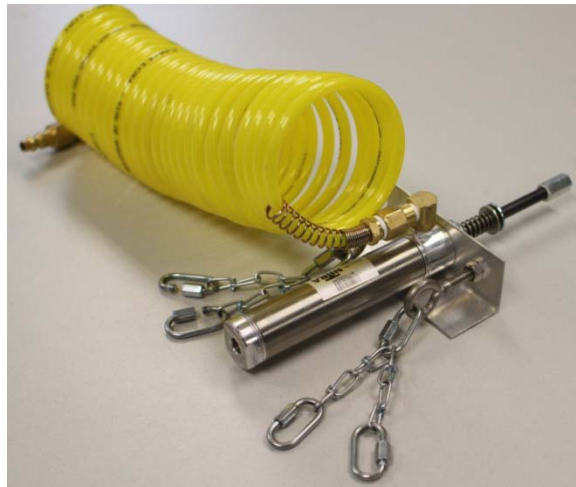
FIG. 5-27. Pneumatic Cylinder Assembly with Nylon Recoil Hose
