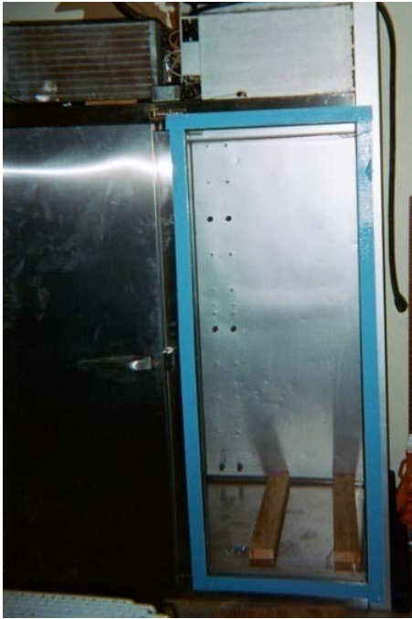
FIG. A-4. Environmental Testing Chamber with a Single Door Removed
