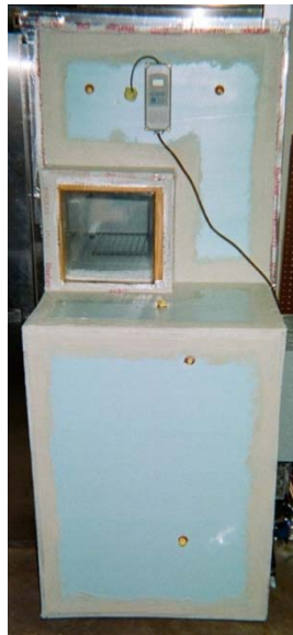
FIG. A-9. Heating Device Rubber Duct Sealant
