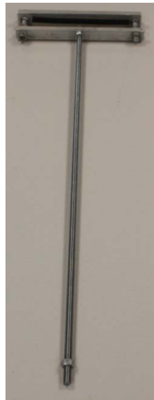
FIG. 5-11. Load Spreading Bar
