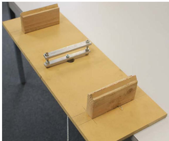
FIG. 5-13. Load Spreading Bar Coupled with Loading Platform
