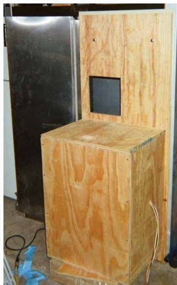
FIG. A-7. Externally Mounted Heating Device Assembly
