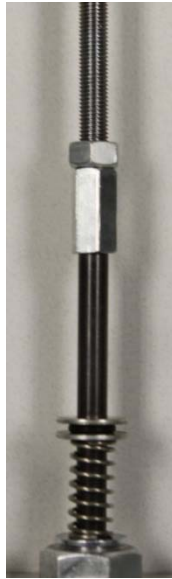
FIG. 5-15. Pneumatic Cylinder Assembly Attachment to Load Spreading Bar through a Coupling Nut
