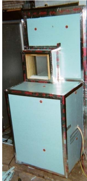
FIG. A-8. Heating Device Insulation and Foil Tape
