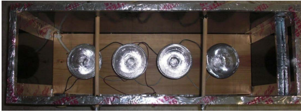
FIG. 5-30. Stress Relief Heating Chamber
