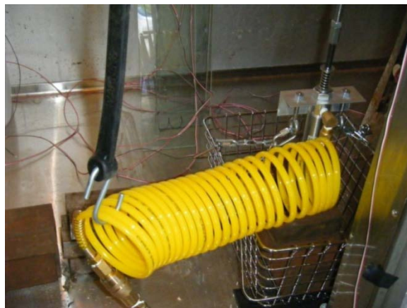
FIG. 5-23. Pneumatic Cylinder Assembly and Weight Basket on Rubber Supports in Environmental Testing Chamber
