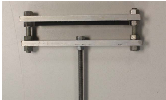
FIG. 5-12. Load Spreading Bar Head Assembly
