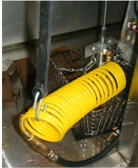
FIG. 5-28. Pneumatic Cylinder Assembly with Nylon Recoil Hose in Environmental Testing Chamber
