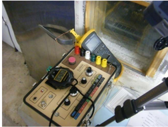
FIG. 5-8. Strain Indicator, Thermocouple Indicator, and Timer Setup
