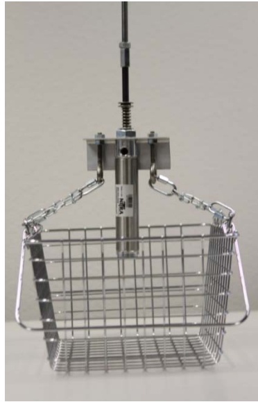
FIG. 5-20. Pneumatic Cylinder Assembly Attached to Weight Basket (Front View)
