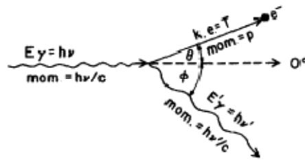
Figure 3. Kinematics of Compton scattering (from Ref. 11).
