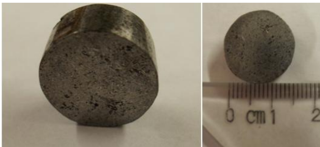
Figure 39 GSG-Al cylindrical sample approximately 16 mm in diameter
