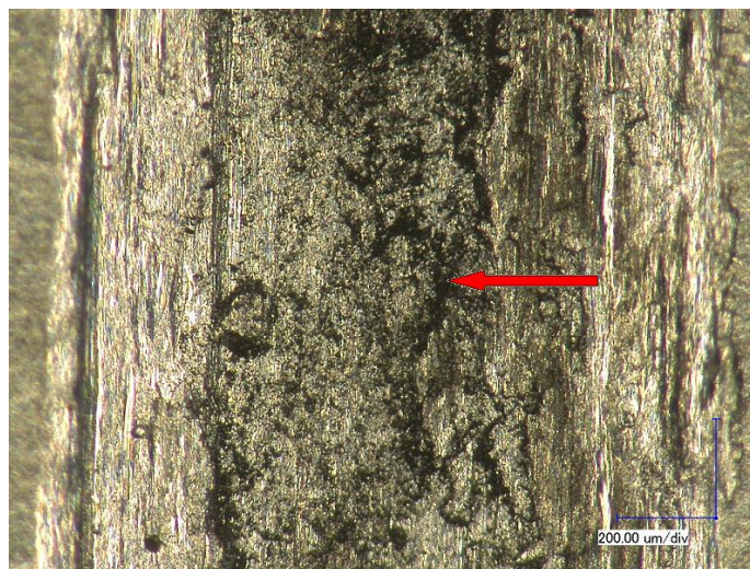
Figure 84 Magnified view (200X) of a wear track of Al 6061-T651 worn at a temperature of 25°C
