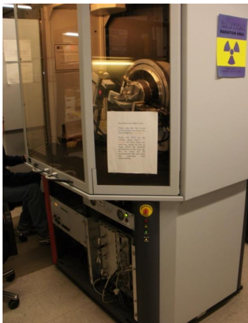
Figure 14 XRD machine used to perform analysis on samples of GSG-Al (housed in the Chemistry Department of Texas A&M University)
