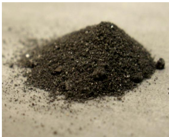
Figure 72 Specimen of GSG after it was affected by many cycles of magnetostriction and phase changes
