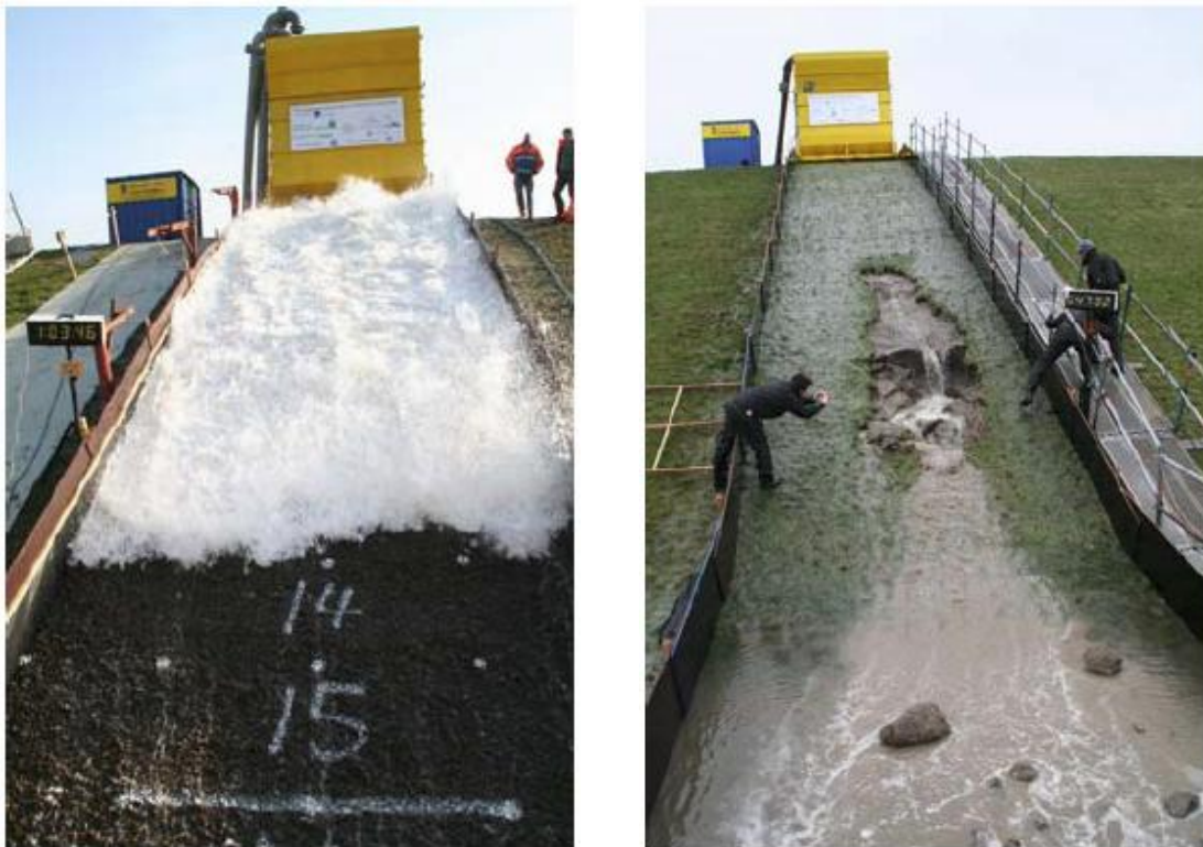
Figure 9. Example of Overtopping Simulator in Action and Erosion Effects (van der Meer et al., 2009).
