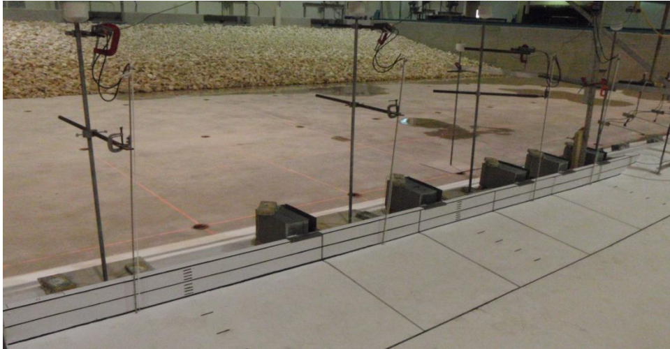
Figure 29. Floodwall Gauge and Overtopping Container Placement.
