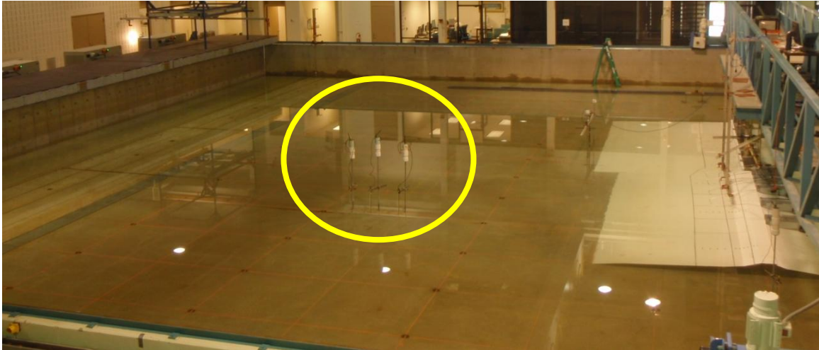
Figure 34. Three-gauge Array Placement.
