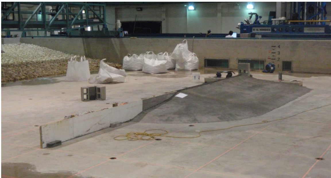
Figure 20. Completed Levee Section of Levee Transition Model.
