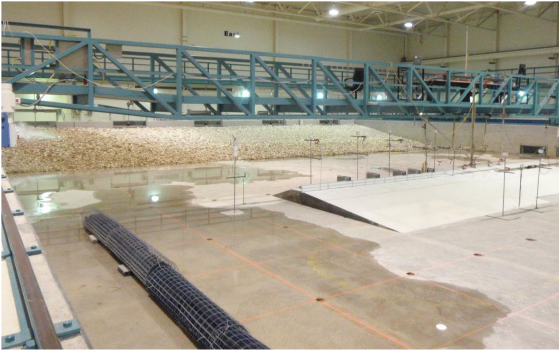
B-1. Floodwall side of modeled levee transition and sidewall absorbers during filling of basin.
