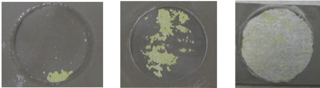
Figure 15 Delamination modes on coating/substrate. (a) failure at stud-coating interface (b) failure at coating (c) failure at coating-substrate
