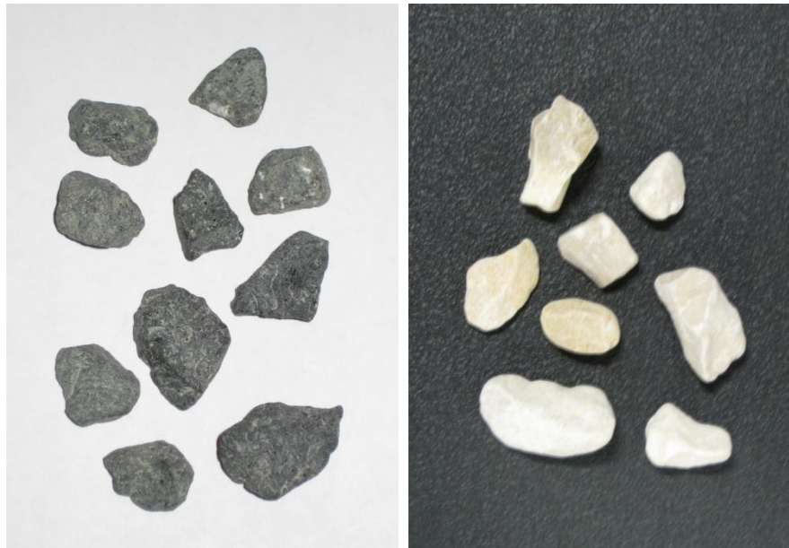
Fig. 4.1. Dark and Light 9.5mm (0.375 in) Aggregates Used in Experiment 1
