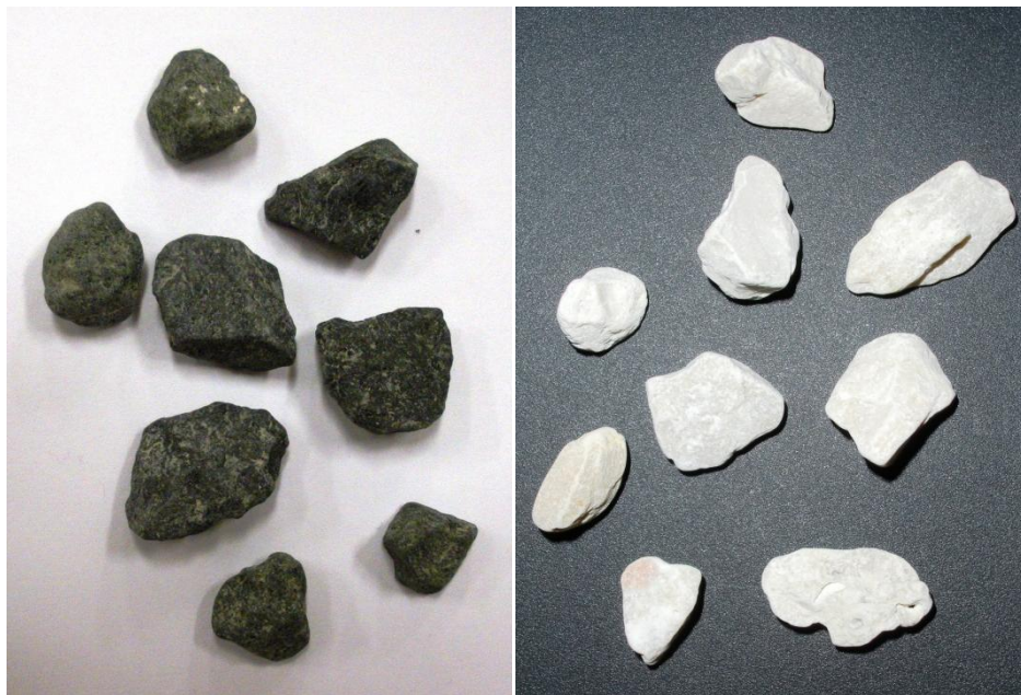
Fig. 4.4. Dark and Light 9.5mm (0.375 in) Aggregates Used in Experiment 5
