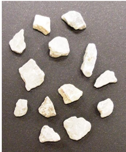
Fig. 4.11. Light 4.75mm (ASTM #4 Sieve) Aggregates Used in Experiment 5
