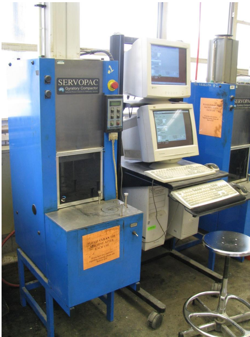
Figure 17. The Superpave Gyrotory Compactor (SGC) Used in This Study
