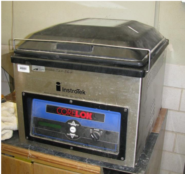
Figure 18. The CoreLok Tester Used to Measure Specimen Specific Gravity
