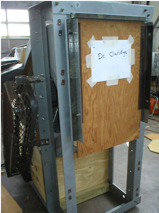
Figure 29: Airflow control used a gate (shown in the closed position).
