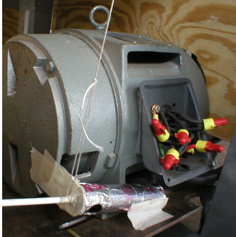
Figure 33: The radiation shield was positioned so that ejected air from the motor blew directly into the intake hole of the radiation shield.
