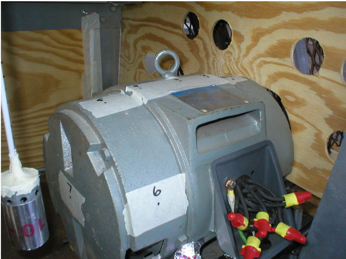
Figure 31: Motor #2 with seven demarcated locations for IR temperature measurement. Masking tape was used in order to reduce errors from mis-specified emissivities. On the left-hand corner is the inside "ambient" air temperature thermometer which was only used for diagnostics.
