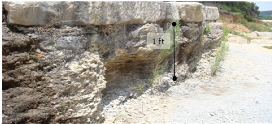
Figure 35. Rock unit 2-10. Unit 2-10 is a heavily clay dominated wackestone that is 2.2 m (7.2 ft) thick.
