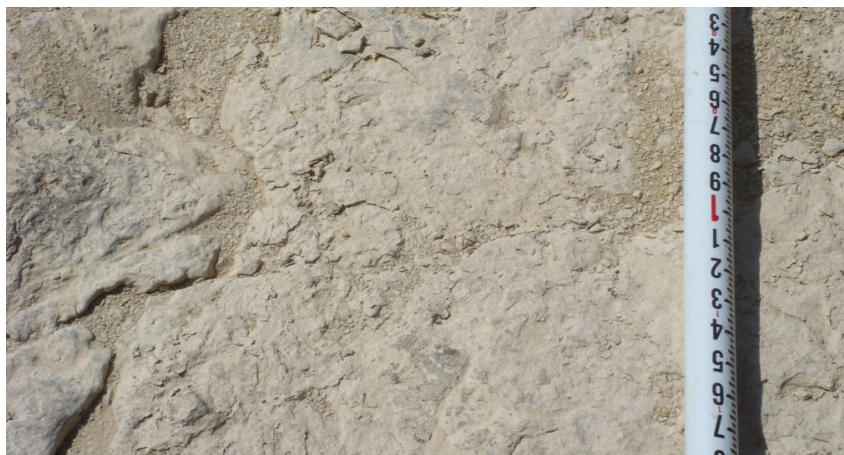
Figure 41. Rock unit 3-2. Unit 3-2 is a packstone that is 0.55 m (1.8 ft) thick. Clay content appears greater than other packstones.
