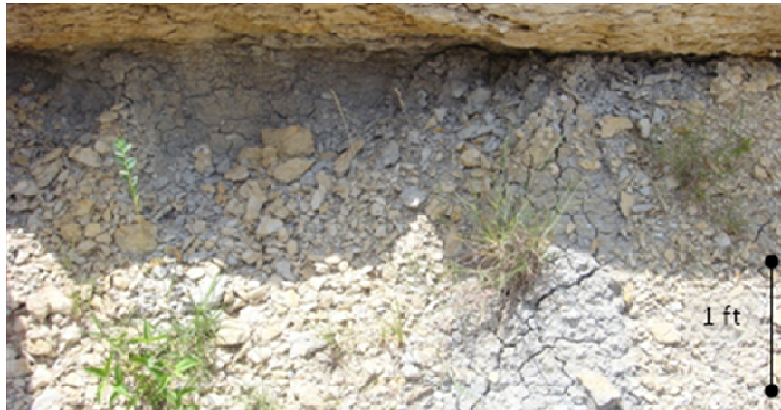
Figure 26. Rock unit 2-1. Unit 2-1 is a wackestone and is 1.28 m (4.2 ft) 1.28 m thick.
