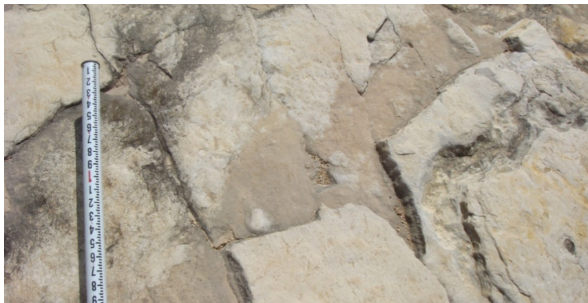
Figure 40. Rock unit 3-1. Unit 3-1 is a packstone that is 0.67 m (2.2 ft) thick. It is consolidated and relatively homogenous in appearance.
