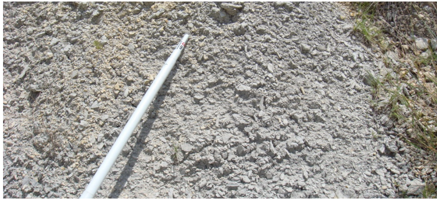
Figure 21. Rock unit 1-1. Unit 1-1 is a wackestone that is 1.04 m (3.4 ft) thick. This rock is very friable, and is seen in this reach creating a slope.
