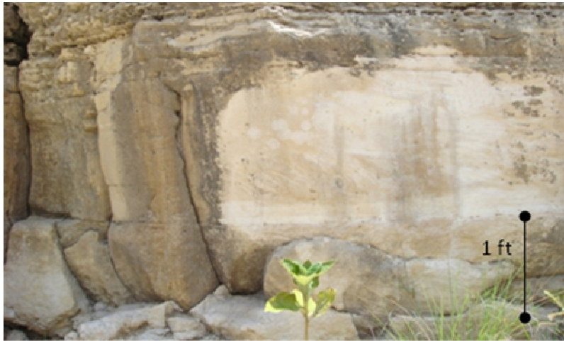
Figure 22. Rock unit 1-2. Unit 1-2 is a homogeneous packstone that is 1.34 m (4.4 ft) thick.
