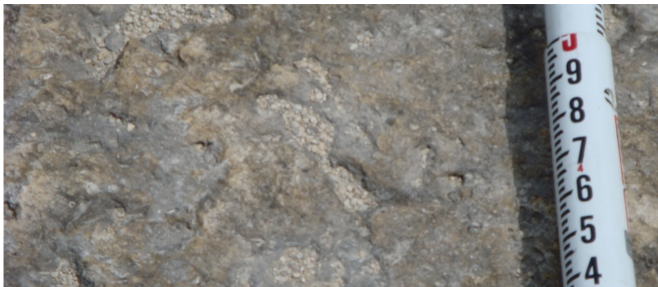
Figure 34. Rock unit 2-9. Unit 2-9 is a homogenous grainstone that is 0.61 m (2.0 ft) thick. This is a very competent unit, and displays vuggy porosity.
