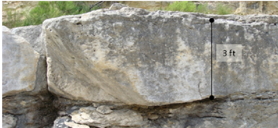
Figure 36. Rock unit 2-11. Unit 2-11 is a homogenous packstone that is 0.95 m (3.1 ft) thick. This unit is a ledge former that is very consolidated and indurated, with sparse vuggy porosity.
