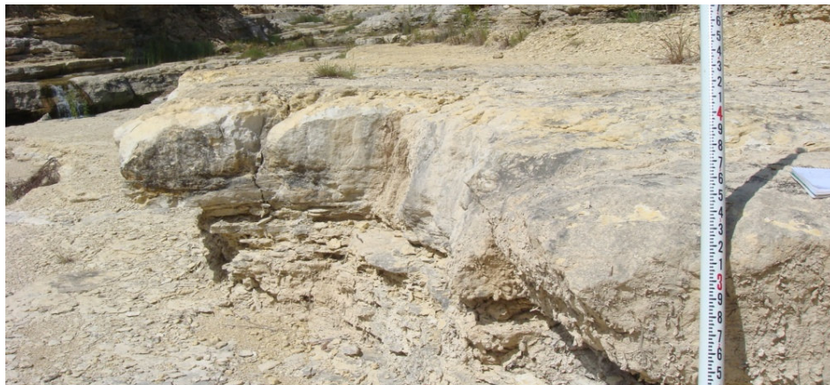
Figure 43. Rock unit 3-4. Unit 3-4 is a packstone that is 0.46 m (1.5 ft) thick. This unit is a consolidated, ledge forming rock.
