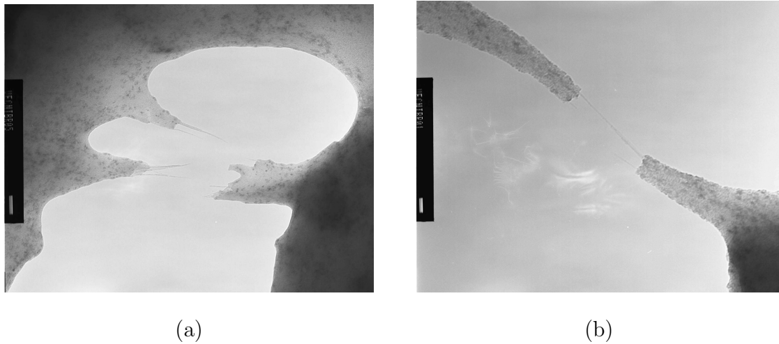
Fig. 15. TEM micrographs showing bridging SWCNTs in epoxy matrix. 15(a) CNTs bridging between matrix surfaces 15(b) Higher magnification image of single bridging CNT (or rope).
