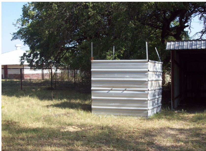
Figure B-2. Burn compartment created for this study, the final product was light-weight and easily transferable within burn treatments.
