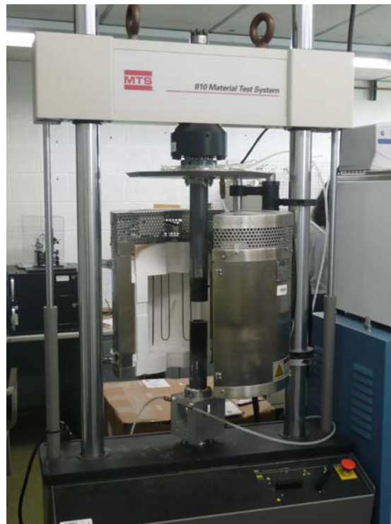
Figure 2.19 MTS 810 Material Test System setup for compression test at (a) room temperature and (b) high temperature
