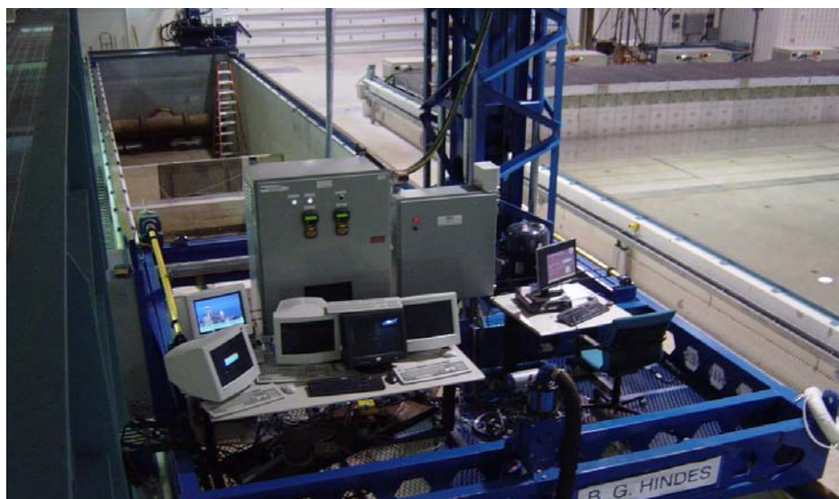
Figure 32. Picture of the Data Acquisition Arrangement of the ADV and OBS Sensors
