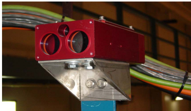
Figure 24. Horizontal Position Laser Mounted on the Dredge/Tow Carriage
