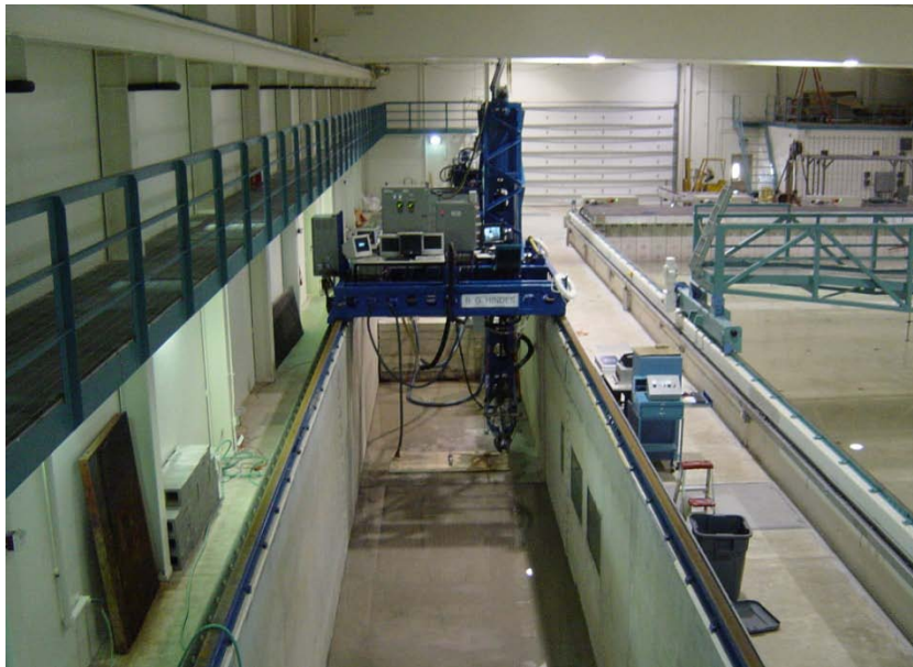
Figure 16. Dredge/Tow Carriage Sitting atop the Dredge/Tow Flume and Sediment Pit
