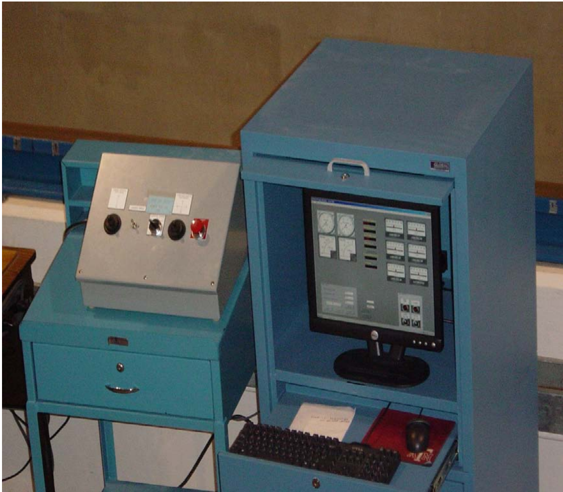
Figure 21. Manual Control System (left) Next to PC Automation System (right)
