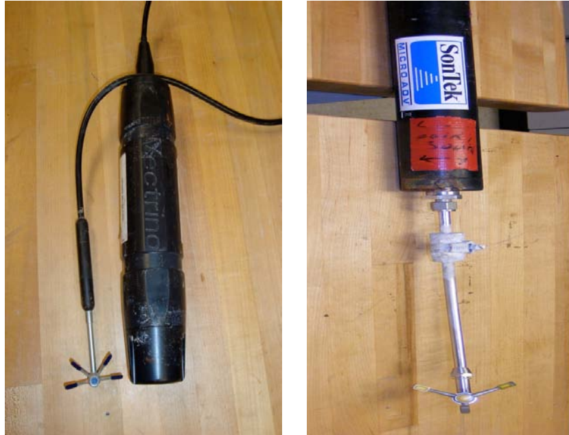
Figure 28. Nortek (left) and Sontek (right) ADV Sensors
