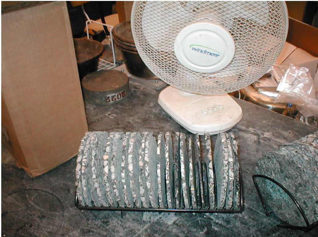
Figure II-4. Core Slices Being Dried
