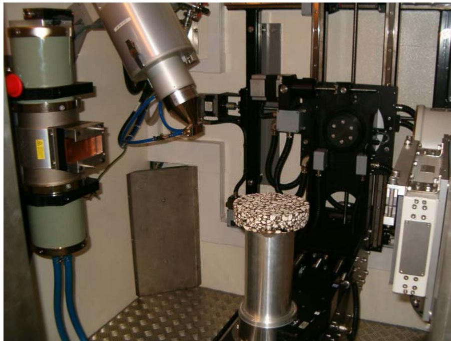
Figure III-1. Specimen Set-Up during X-Ray CT Scanning
