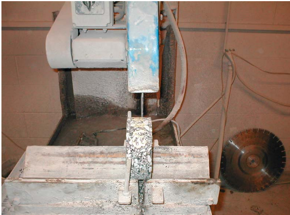
Figure II-3. Slicing Cores for Further Testing
