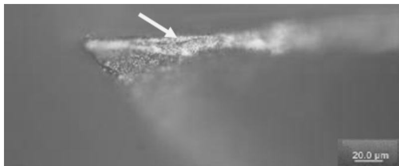
Figure 34: Optical microscope generated image of coating chip off (shown by arrow) on a TiN coated end-mill (mist cooling/lubrication, machining time: 246s; cutting speed: 0.08m/min).
