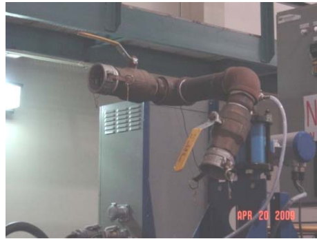
Figure 17: Two way valve, with the nuclear density gauge and flowmeter attached to it.
