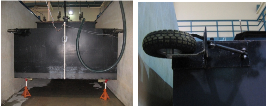
Figure 5: Hopper barge resting on jacks (left) rubber tires act as fenders (right).
