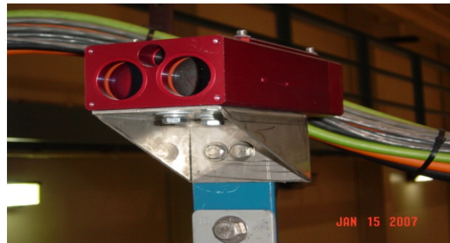
Figure 15: Picture of the horizontal position laser mounted on the dredge/tow carriage.
