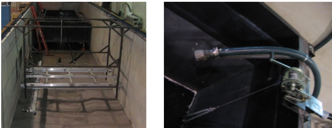
Figure 22: Laser Profiler on the frame, hanging from the top of the tow tank (left) Hose attached to the hopper barge (right).
