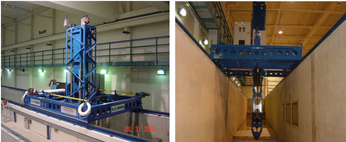
Figure 2: Different views of carriage mounted on the rails of the tow tank with cutter seen in the bottom (right).
