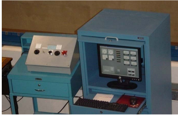
Figure 12: Manual control system (left) next to PC automation system (right).
