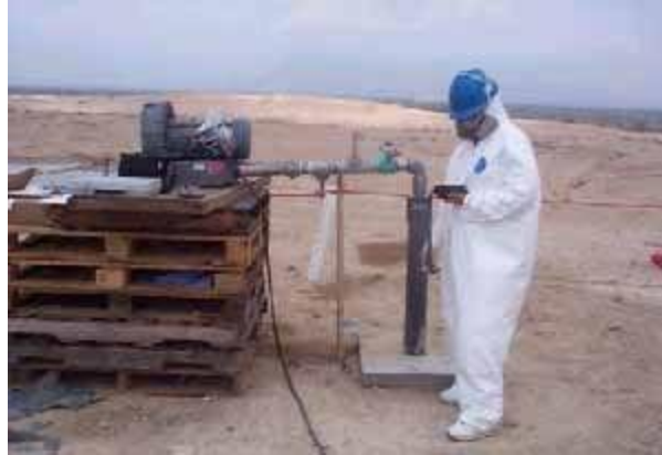
Figure 20: Operator Performing a Pump Test (World Bank 2002)
