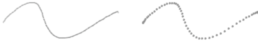
Figure 3. Example of a digitized stroke. When a curve is drawn on a digitizing surface (left), the movement is sampled as data points with coordinates and a time (right).
