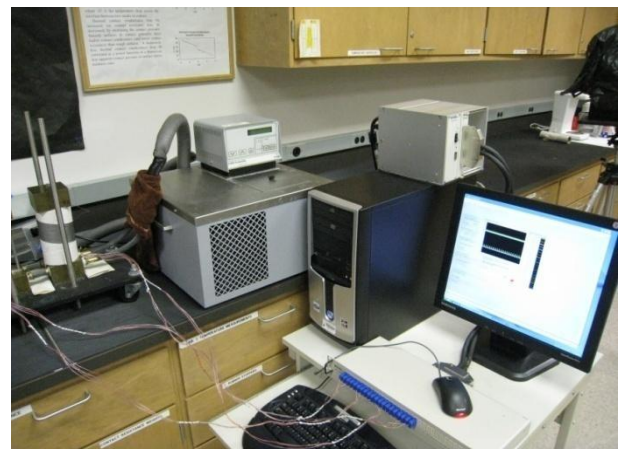
Fig. 2.7 Experimental setup. Stainless steel rod and thermocouples
