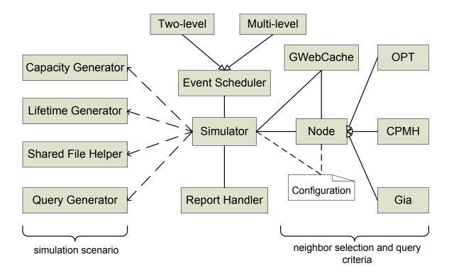
Fig. 3. Architecture of POSIM.
