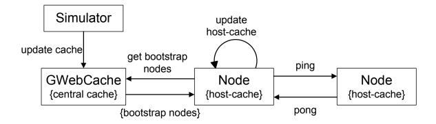
Fig. 6. Bootstrap mechanism in POSIM.
