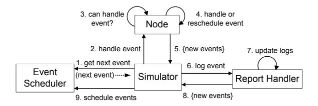
Fig. 4. Event handling mechanism in POSIM.
