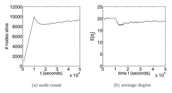
Fig. 13. Evolution of CSOD-CPMH network under churn.
