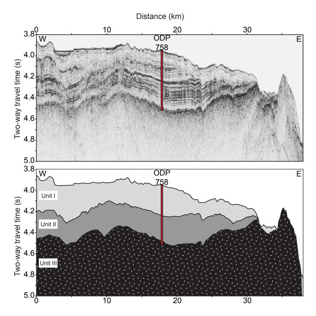
Figure 4. Seismic Reflection Profile from KNOX06RR Site 758. Uninterpreted version (top) and interpreted version (bottom) showing the division into three Seismic Units I, II, and III. Vertical red bar indicates approximate location and depth of ODP Site 758.
