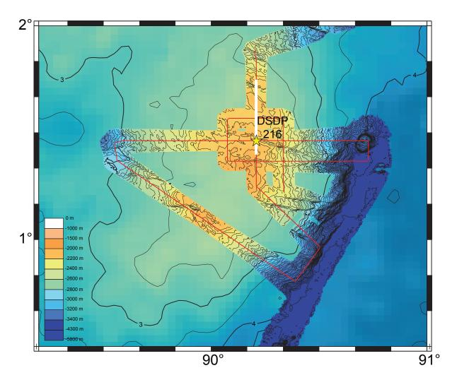
Figure 5. Seisimic Survey Map of KNOX06RR Site 216. Tracklines are shown in red. White bar indicates location of seismic profile in Figure 7. Star indicates location of DSDP Site 216. Multibeam bathymetry data are overlaid on predicted bathymetry (after Smith and Sandwell, 1997). Colors indicate depth with blue being deepest and warm colors shallowest. Multibeam bathymetry contour interval = 50 m. Predicted bathymetry contour interval = 500 m.
