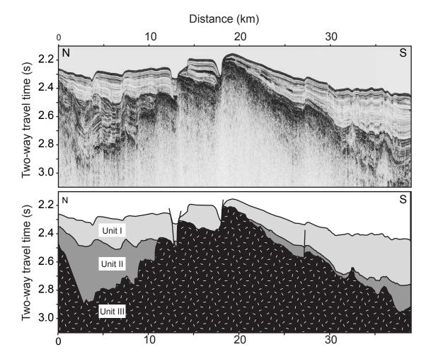
Figure 21. Seismic Reflection Profile from KNOX06RR Site 253. Conventions as in Figure 4.
