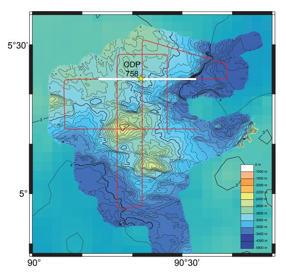
Figure 2. Seismic Survey Map of KNOX06RR Site 758. Tracklines are shown in red. White bar indicates location of seismic profile in Figure 4. Star indicates location of ODP Site 758. Multibeam bathymetry data are overlaid on predicted bathymetry (after Smith and Sandwell, 1997). Colors indicate depth with blue being deepest and warm colors shallowest. Multibeam bathymetry contour interval = 100 m. Predicted bathymetry contour interval = 100 m.
