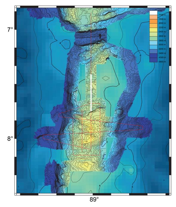
Figure 11. Seismic Survey Map of KNOX06RR Site NER3. Tracklines are shown in red. White bar indicates location of seismic profile in Figure 13. Conventions as in Figure 5.
