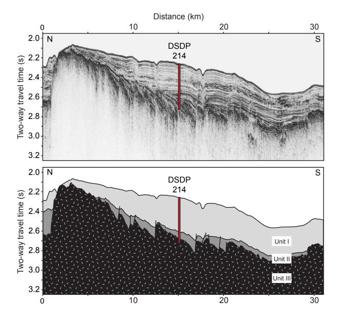
Figure 16. Seismic Reflection Profile from KNOX06RR Site 214. Conventions as in Figure 4.
