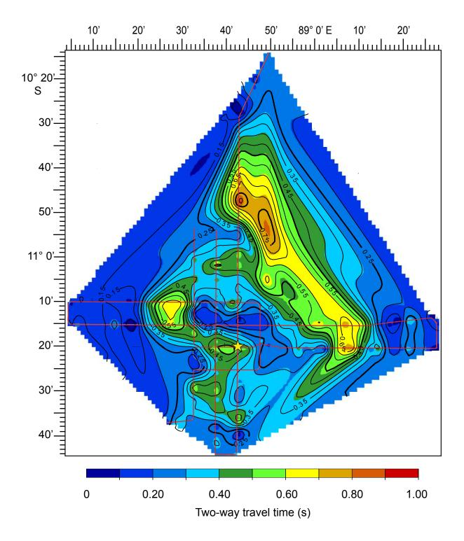
Figure 15. Total Sediment Thickness Isopach Map of KNOX06RR Site 214. Star indicates location of DSDP Site 214. Conventions as in Figure 3.
