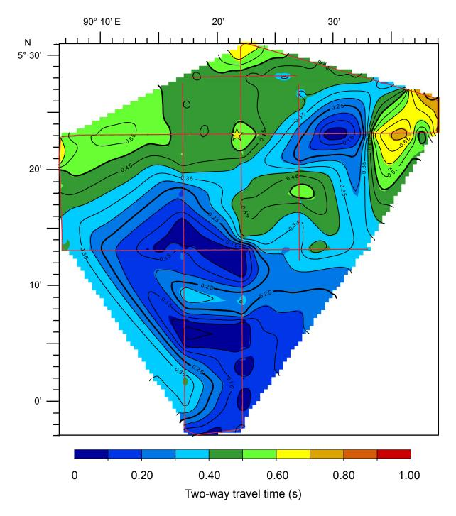
Figure 3. Total Sediment Thickness Isopach Map of KNOX06RR Site 758. Isopach represents thickness of sediment column in two-way travel time (s) between seafloor horizon and acoustic basement horizon. Contour interval = 0.05 s. Survey tracklines shown in red. Star indicates location of DSDP Site 758.
