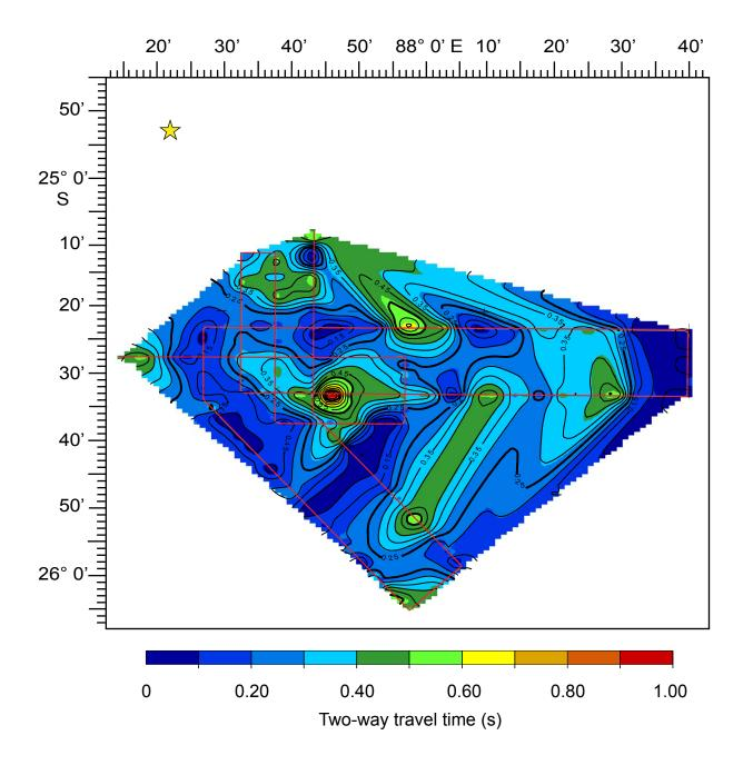
Figure 20. Total Sediment Thickness Isopach Map of KNOX06RR Site 253. Star indicates location of DSDP Site 253. Conventions as in Figure 3.
