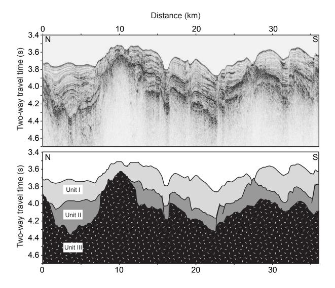
Figure 13. Seismic Reflection Profile from KNOX06RR Site NER3. Conventions as in Figure 4.
