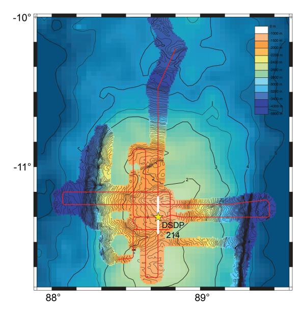
Figure 14. Seismic Survey Map of KNOX06RR Site 214. Tracklines are shown in red. White bar indicates location of seismic profile in Figure 16. Star indicates location of DSDP Site 214. Conventions as in Figure 5.
