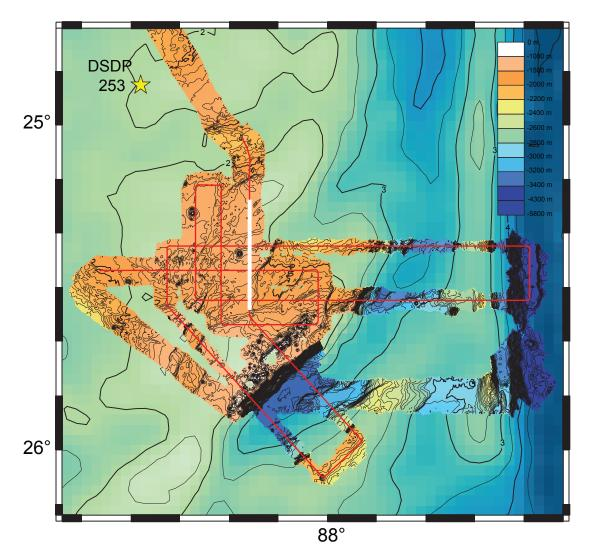
Figure 19. Seismic Survey Map of KNOX06RR Site 253. Tracklines are shown in red. White bar indicates location of seismic profile in Figure 21. Star indicates location of DSDP Site 253. Conventions as in Figure 5.
