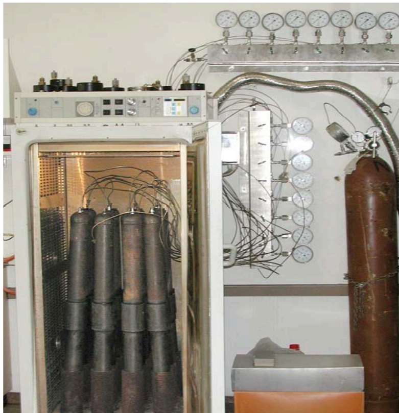
Fig. 32 – Picture of test apparatus showing simulated pipe connection 3
