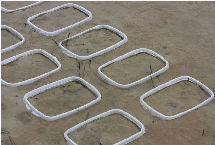
Figure 13: Set-up for Experiment #2. Photograph of the plot enclosures placed on the sediment. Four plots for each treatment were randomly placed in to the sediment into 2 rows of 8 plot enclosures.
