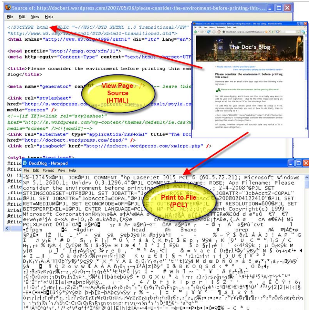
Figure 56: HTML (top) formats content for display by a Web browser; PCL (bottom) formats the same content for a printer.
