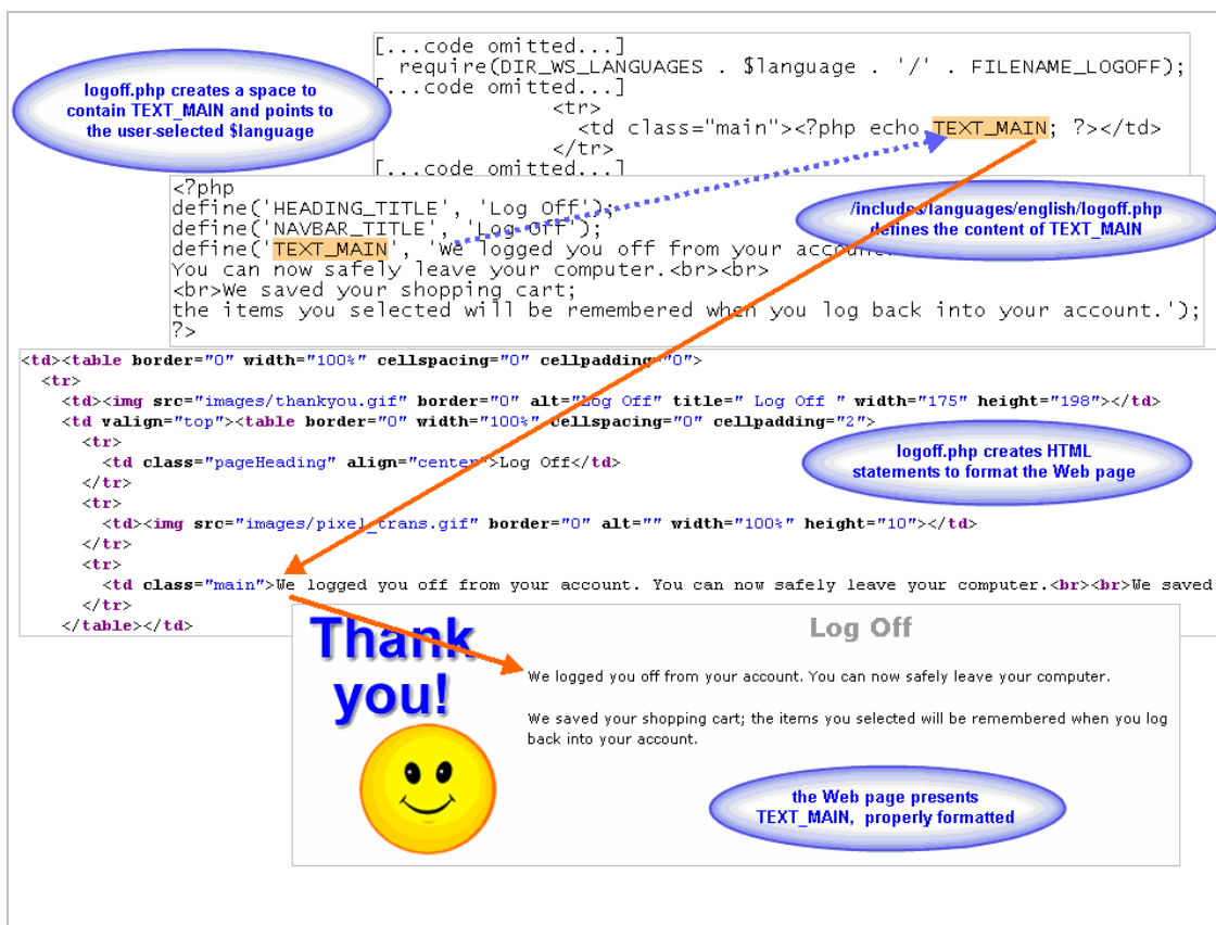
Figure 49: Multiple layers of substitution into placeholders allow human language to be presented with other user-specific data.
