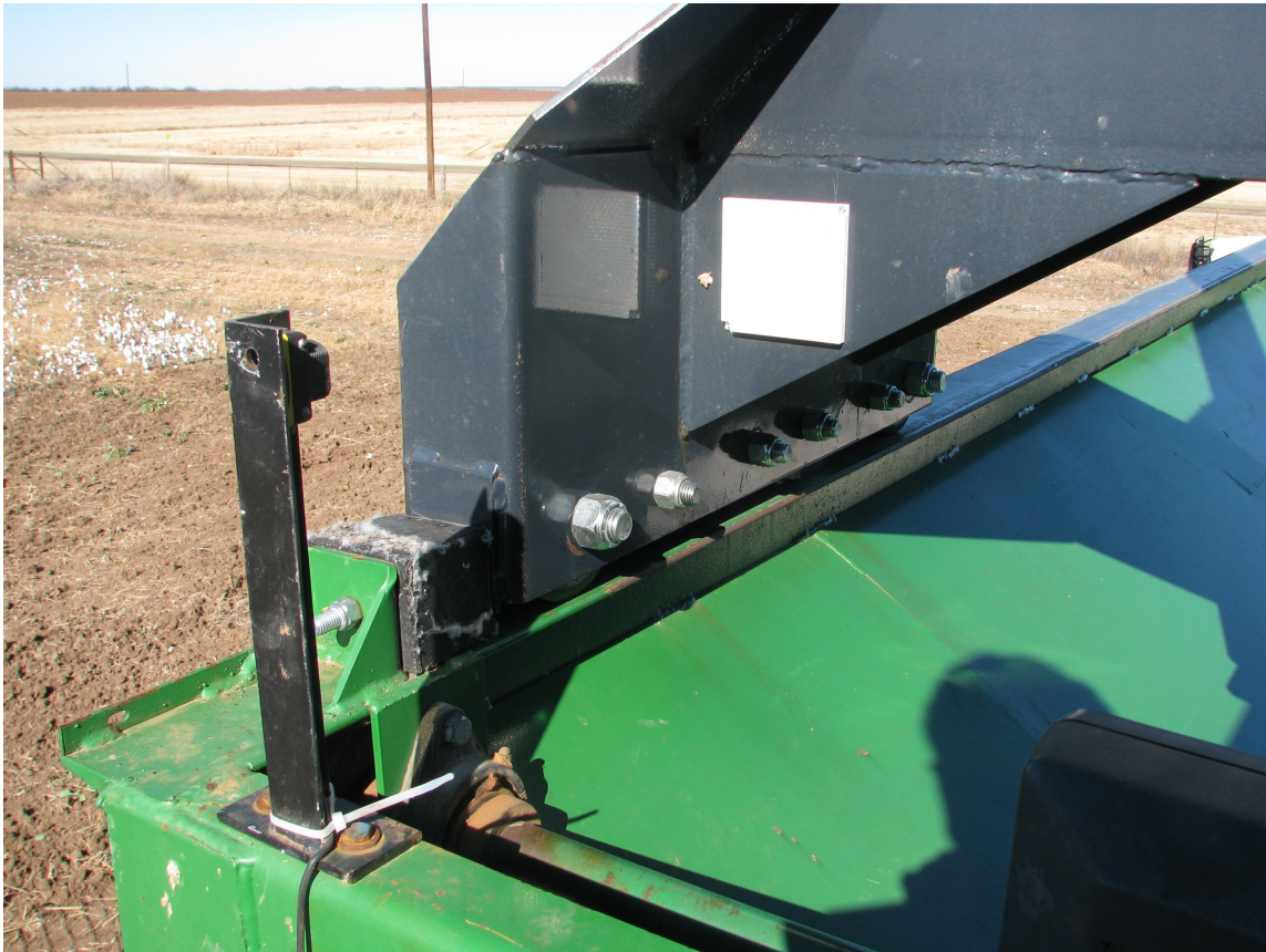
Figure 6.2. Photoelectric sensor and reflector for detecting cotton on sides of module builder.
