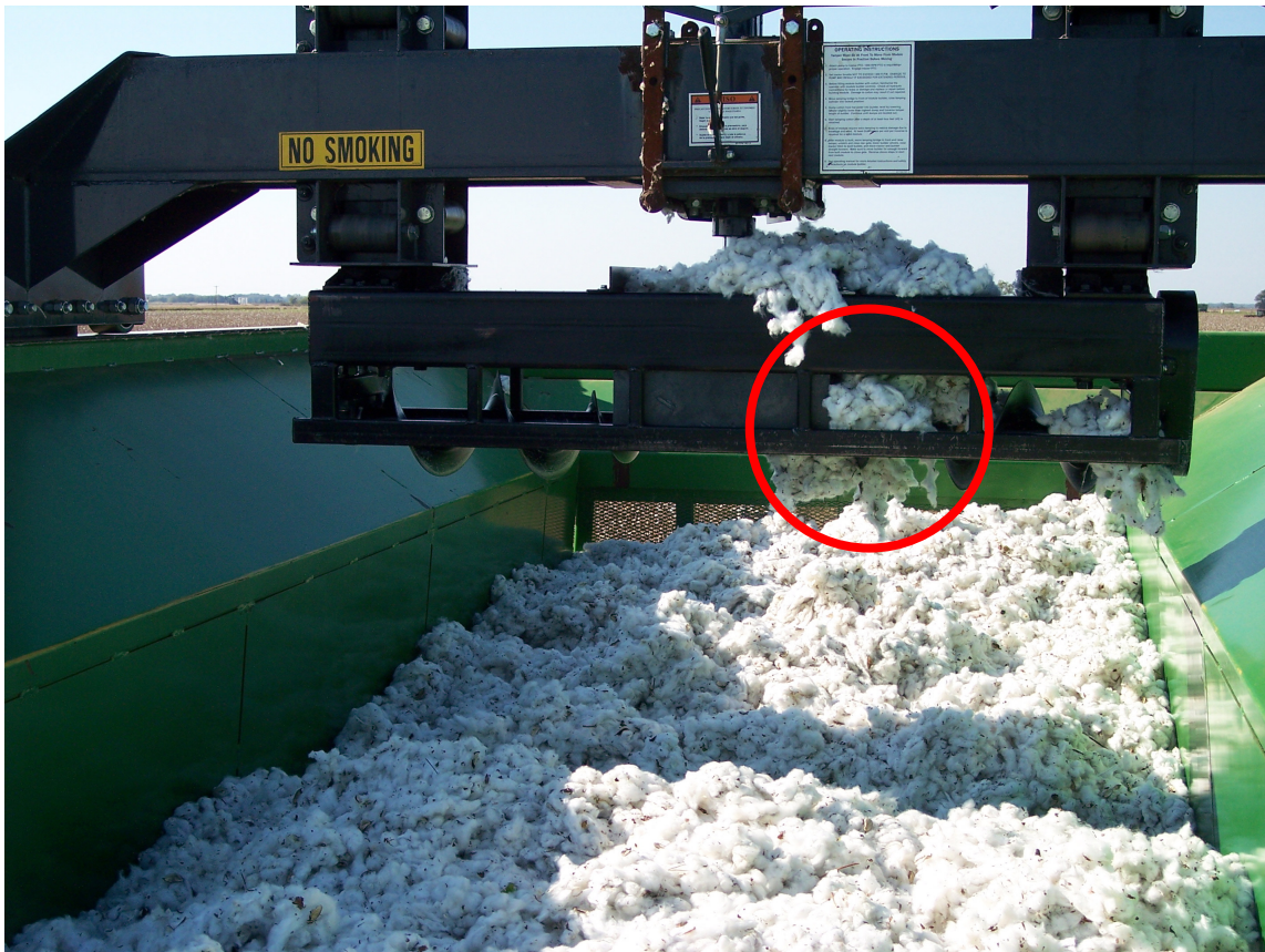
Figure 5.8. Cotton caught in auger housing after tramping stroke.
