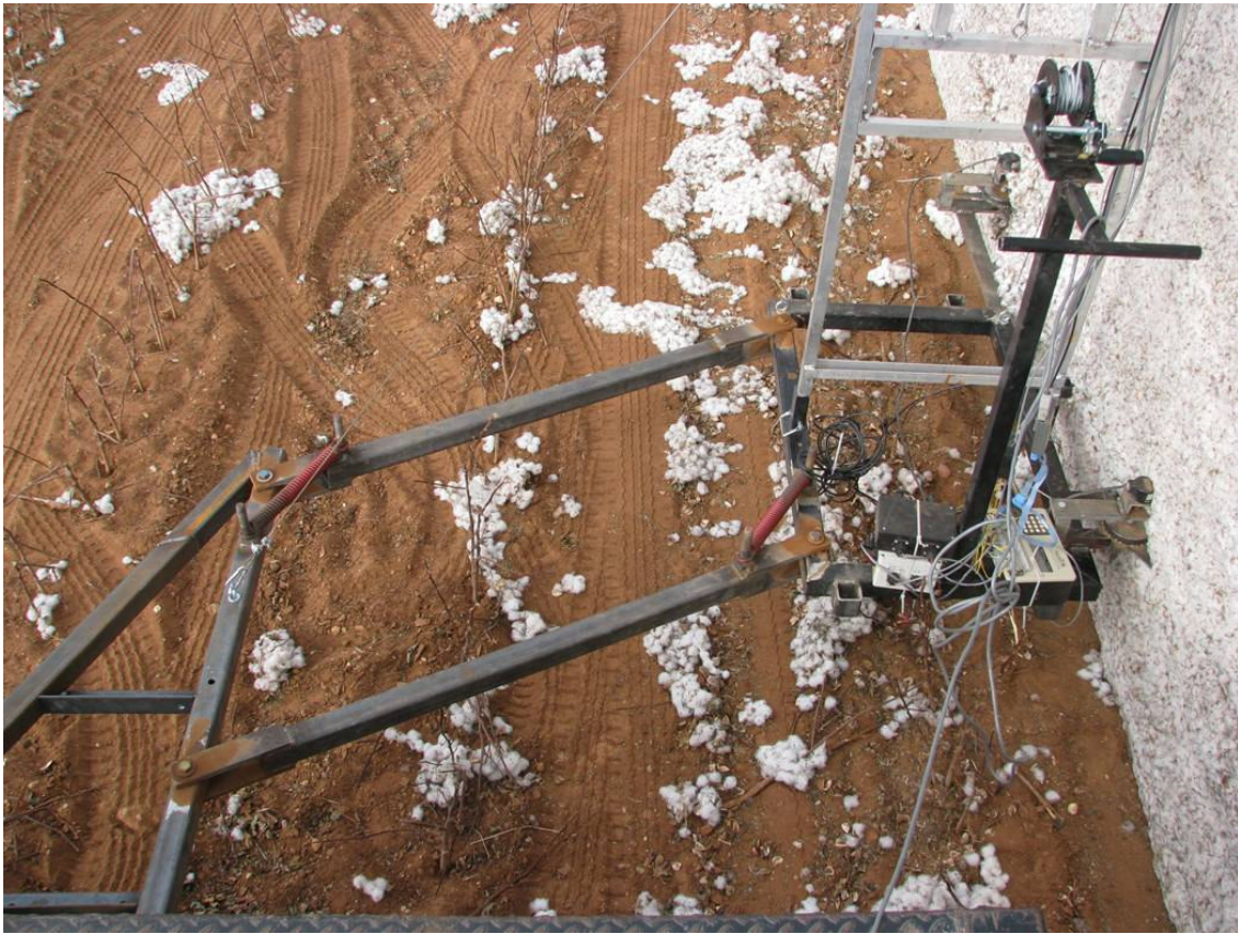
Figure 4.1. Parallel linkages and position sensing apparatus.
