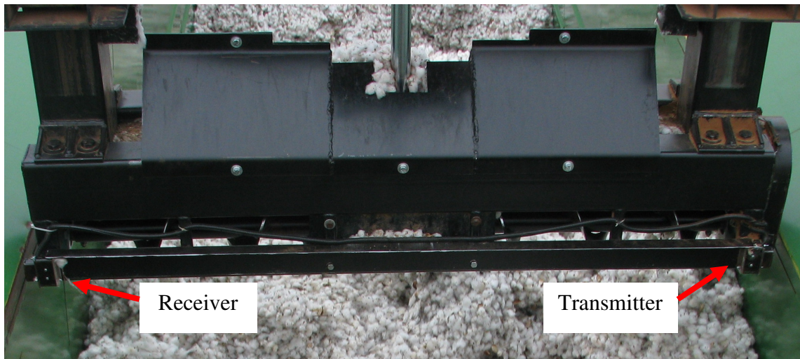
Figure 6.1. Tramper photoelectric sensor. This sensor pair was duplicated on the back side of the tramper.
