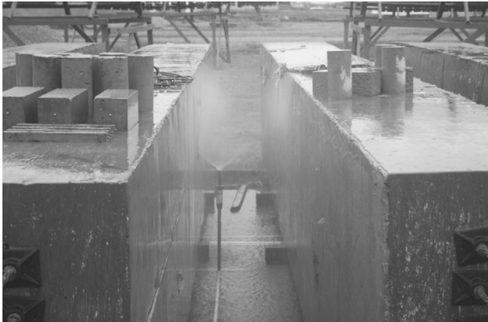
Figure 3-2 Sprinkler System between Two Specimens
