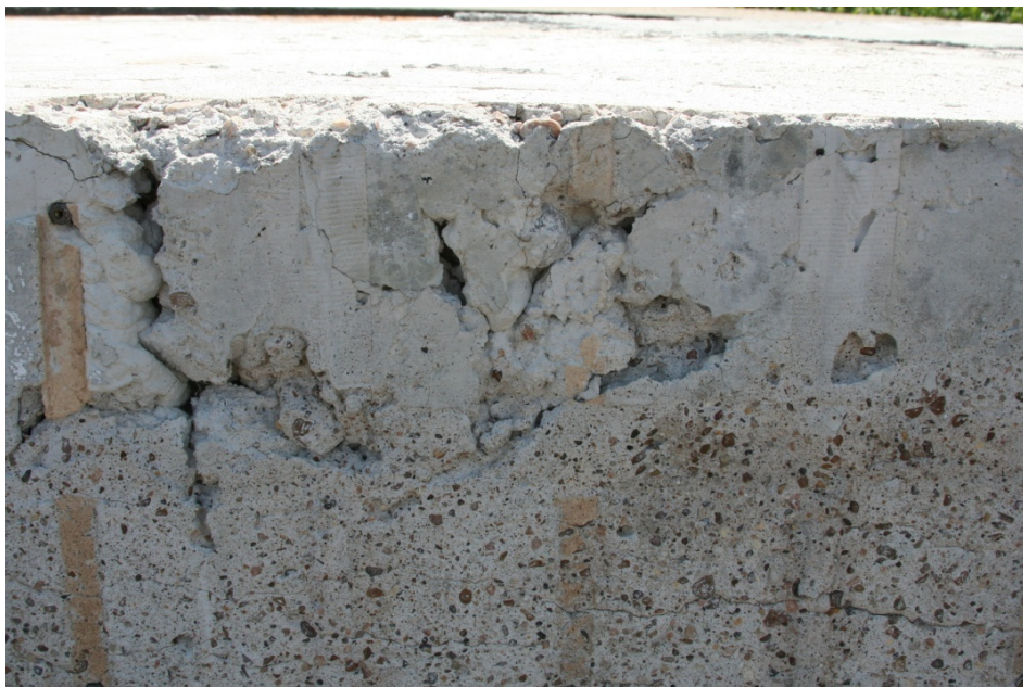
Figure 2-20 Voids in the First Trials
