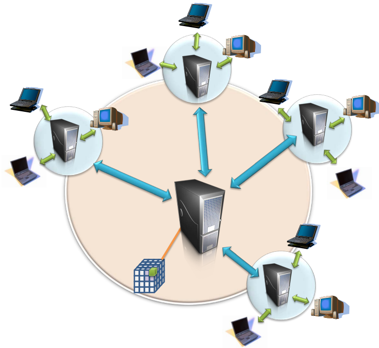
Fig. 43. Mutl-server Configuration. The main server has multiple sub-server and each sub-server manages client connections.
