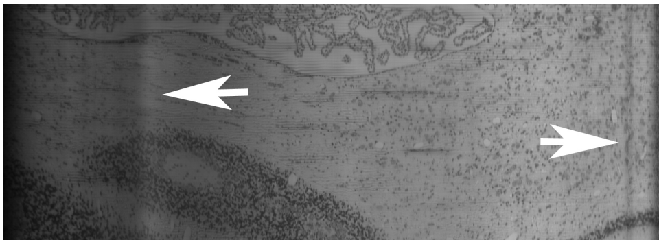
Fig. 21. Overall Intensity Shift. The overall intensity shift along the x -axis is due to knife misalignment (arrows). Adapted from [49].
