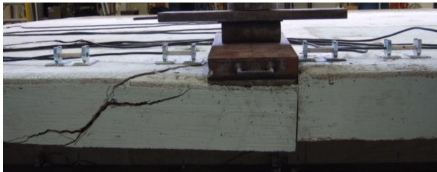
(d) Load Case 2.7: Lab-cast overhang loaded at panel-to-panel seam
