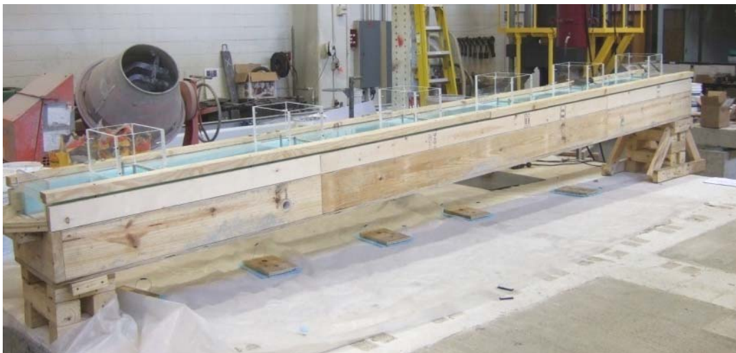
Fig. 32. Experimental grout track on 4% slope
