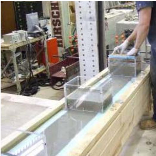
c) Placing grout cover on first pocket
