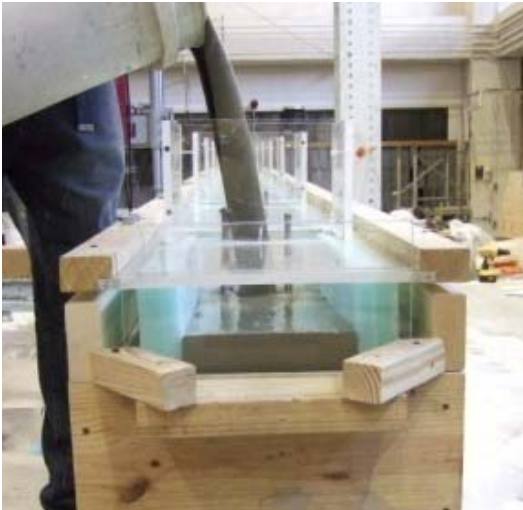
a) Pouring grout in first pocket
