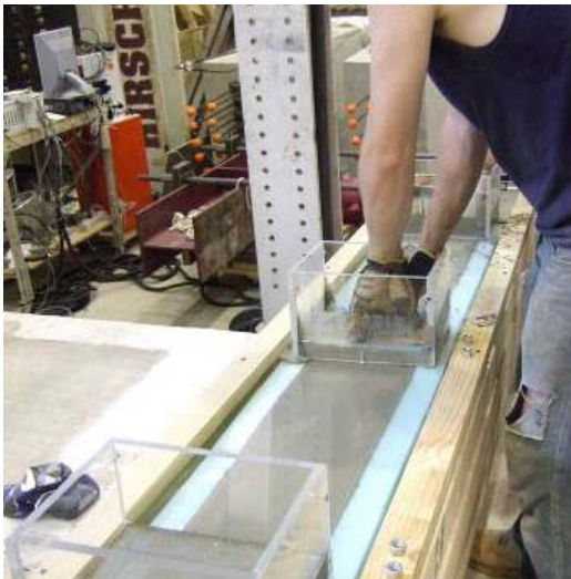
d) Placing grout cover on second pocket
