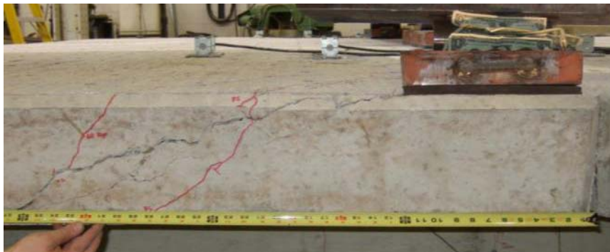
(b) Load Case 1.6: Precast prestressed overhang loaded at panel-to-panel seam
