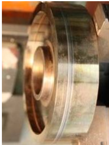
Figure E2: Surface roughness versus axial length of the test discs after ~20 hours of use with side view of shaft and disc. Disc for HBS and brush seal with OD of 165.48 mm and 166.81 mm, respectively.
