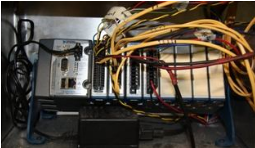
Figure C1: FPGA board with analog inputs, analog outputs, and thermocouples wired.
