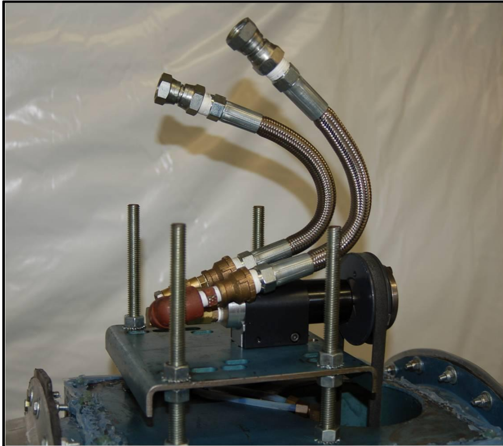
Fig. 2.13 Pneumatic motor and hardware
