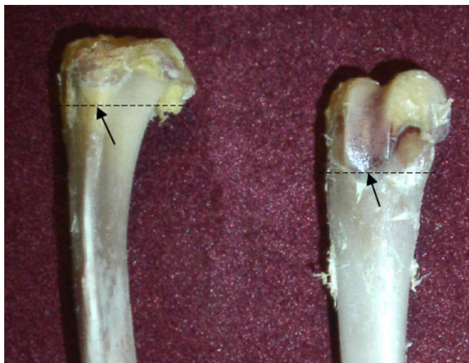
Figure 8: The External Landmarks Chosen as RPC Specimen First Cut Locations for the Tibia (left) and Femur (right) (18)
