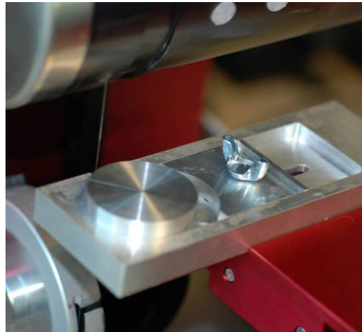
Figure D3: Coring Set Up with Alignment Block
