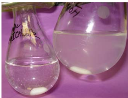
Figure V-1. Schlenk flasks containing the reaction mixtures from synthetic route (b) on the left and route (b') on the right were photographed against a colored background to highlight the clear and cloudy makeup of each colorless solution.
