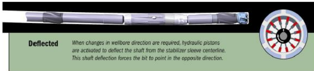
Fig. F.3—Illustrates deflection in the bottom hole assembly (Logging While Drilling 2008).
